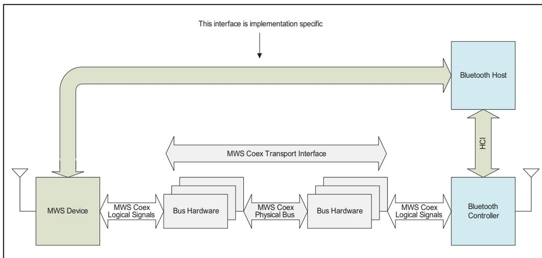
Figure 1.1: Coexistence signaling/messaging architecture
