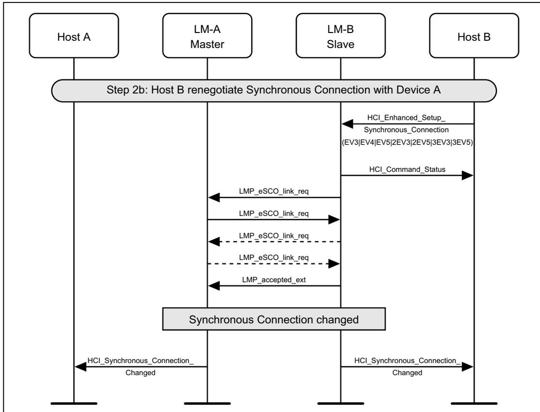
Figure 5.15: Slave renegotiates synchronous connection parameter change
