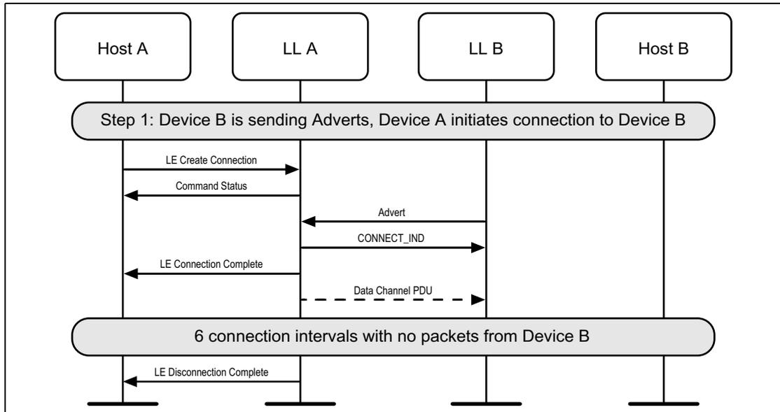
Figure 5.5: Initiating a Connection that fails to establish
