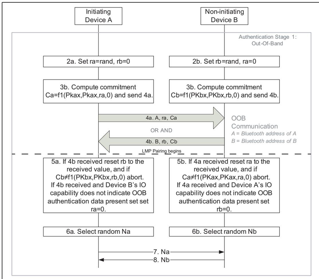
Figure 7.5: Authentication Stage 1: Out of Band Details
