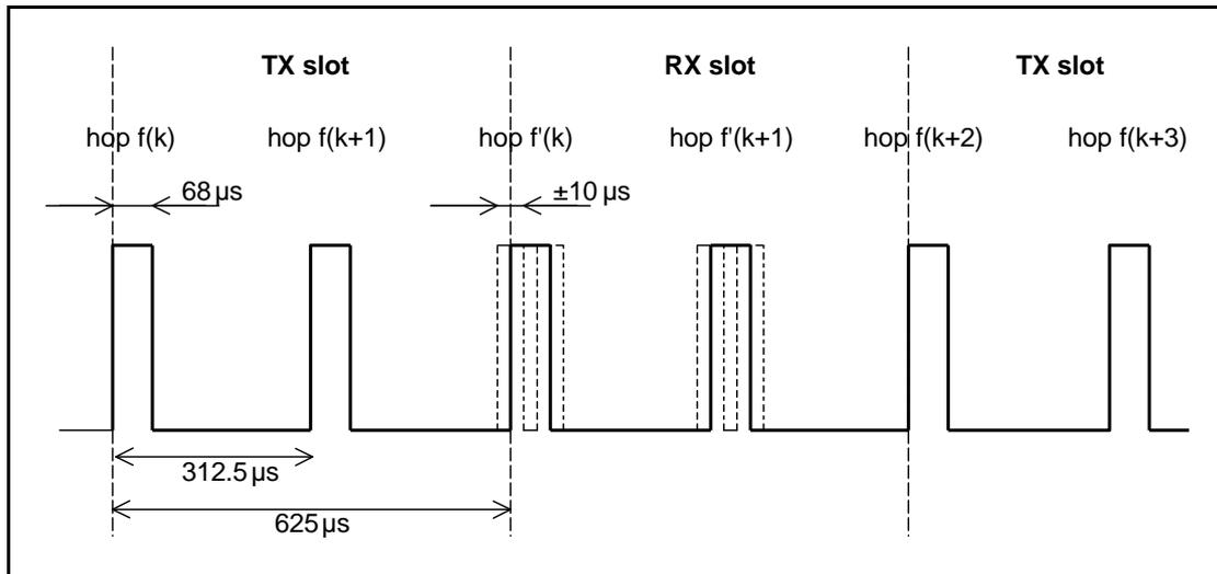
Figure 2.7: RX/TX cycle of transceiver in PAGE mode
