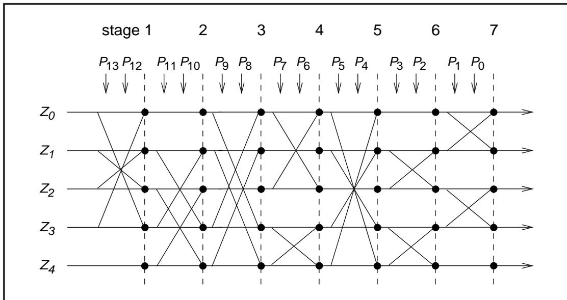
Figure 2.18: Permutation operation for the hop system
