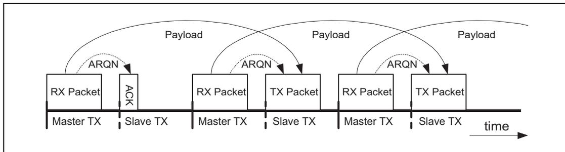
Figure 1.8: Payload & ARQN handling in delayed loopback - start.
