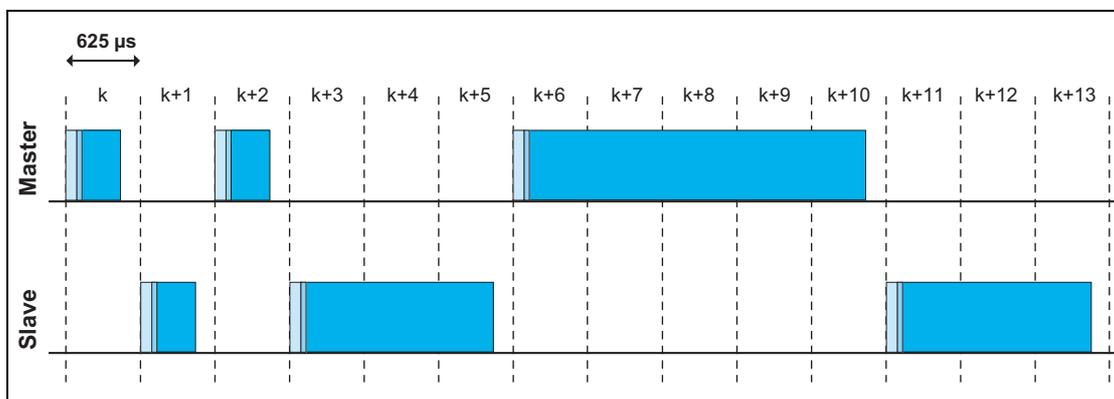
Figure 2.1: Multi-slot packets
