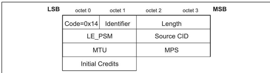
Figure 4.24: LE Credit Based Connection Request Packet
