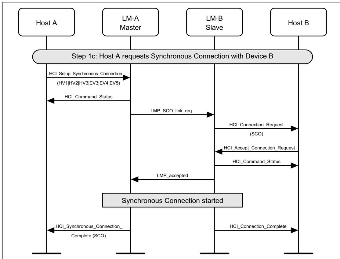
Figure 5.3: Master requests synchronous connection using SCO
