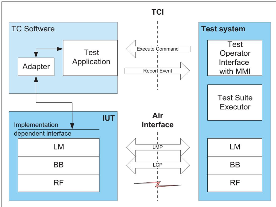
Figure 2.4: BB and LM qualification with “software bearer”
