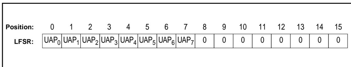
Figure 7.7: Initial state of the CRC generating circuit
