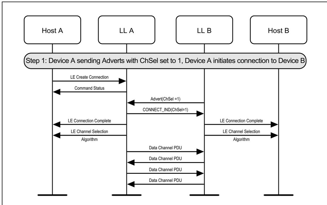
Figure 5.7: Initiating a Channel Selection Algorithm #2 Connection
