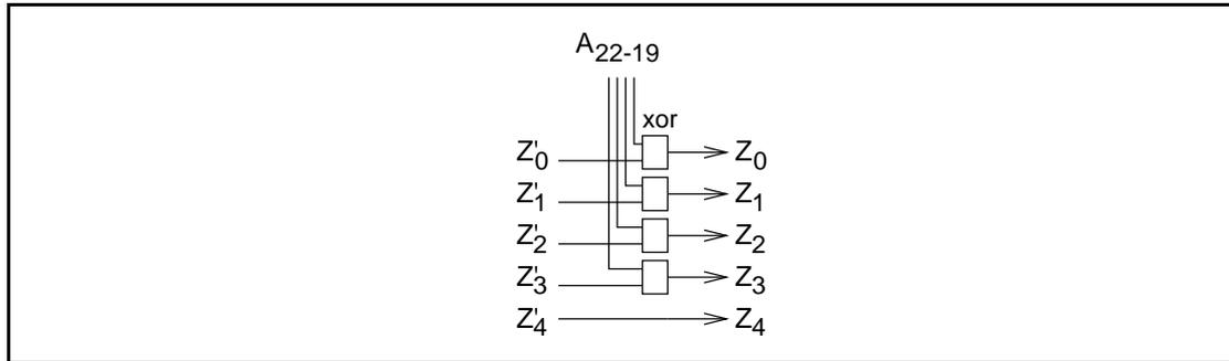
Figure 2.17: XOR operation for the hop system
