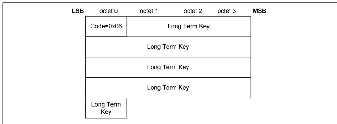
Figure 3.12: Encryption Information Packet
