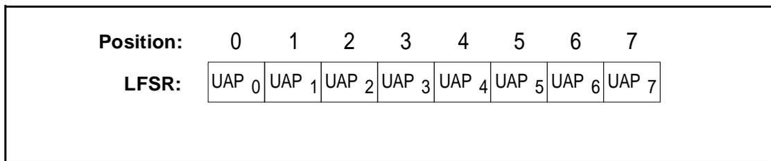
Figure 7.4: Initial state of the HEC generating circuit
