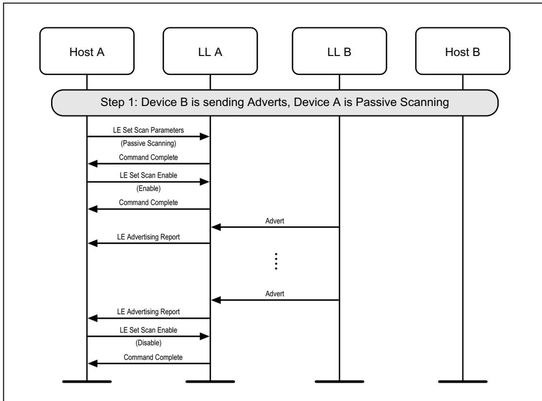
Figure 4.1: Passive Scanning
