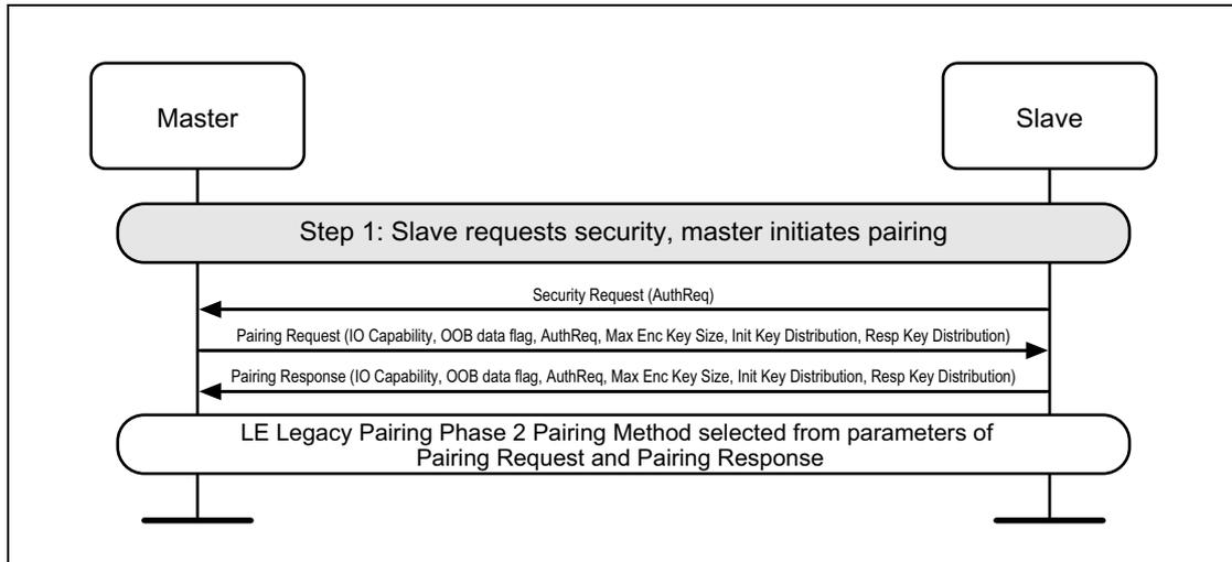
Figure C.3: Slave security request, master initiated pairing
