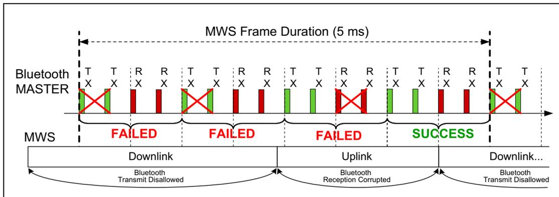
Figure 7.4: Bluetooth radio can suffer Inquiry/Page failures
