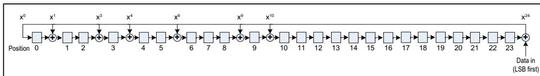
Figure 3.3: The LFSR circuit generating the CRC
