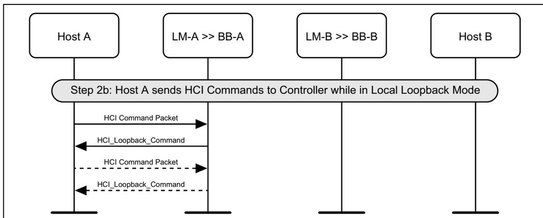
Figure 8.3: Looping back commands in local loopback mode
