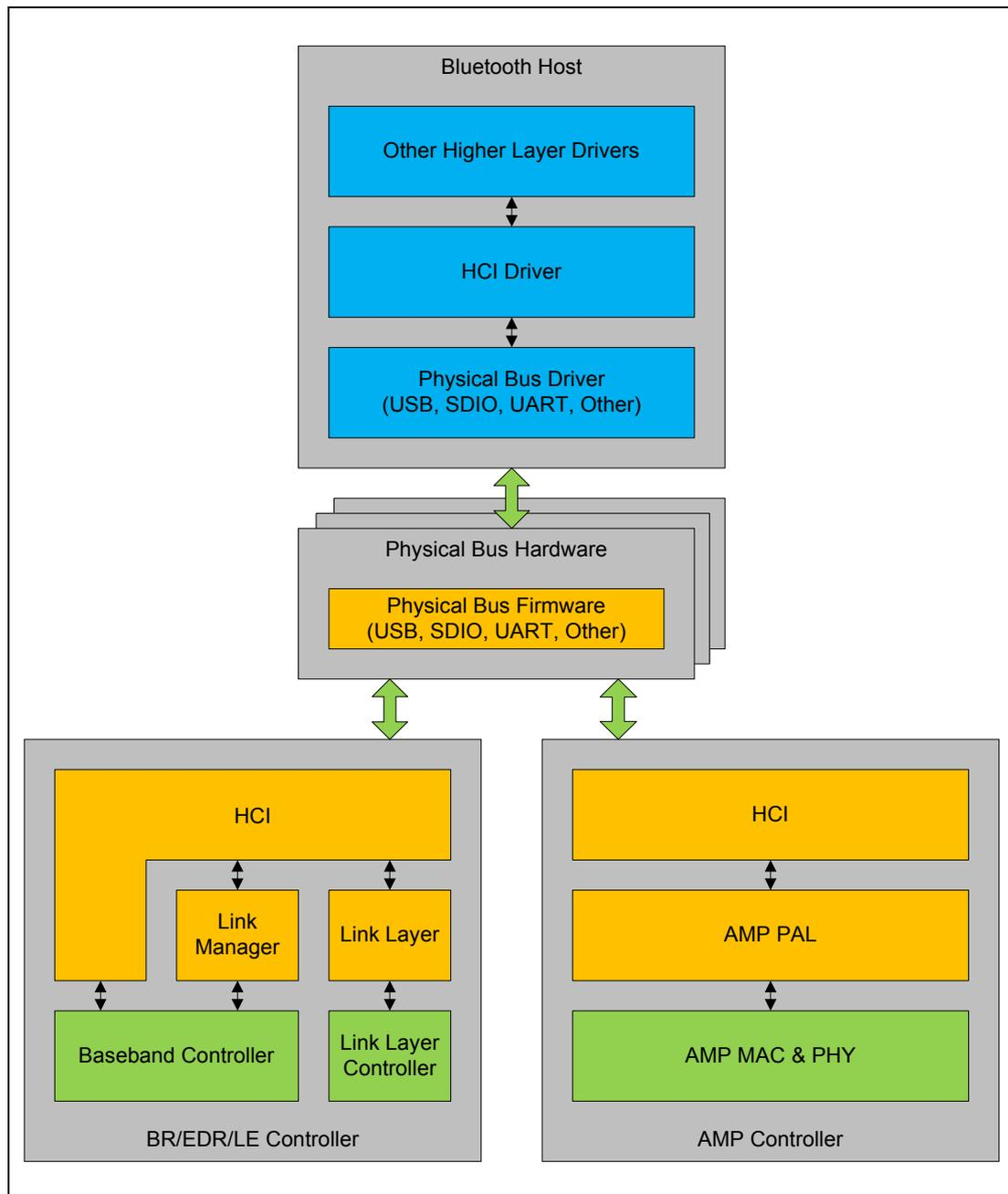
Figure 1.1: Overview of the Lower Software Layers
