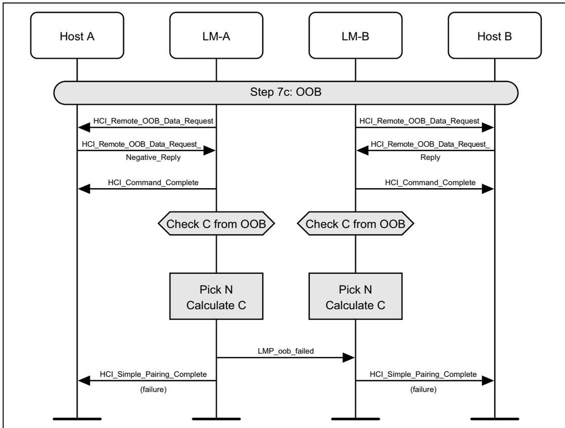
Figure 4.22: OOB authentication failure on initiating side
