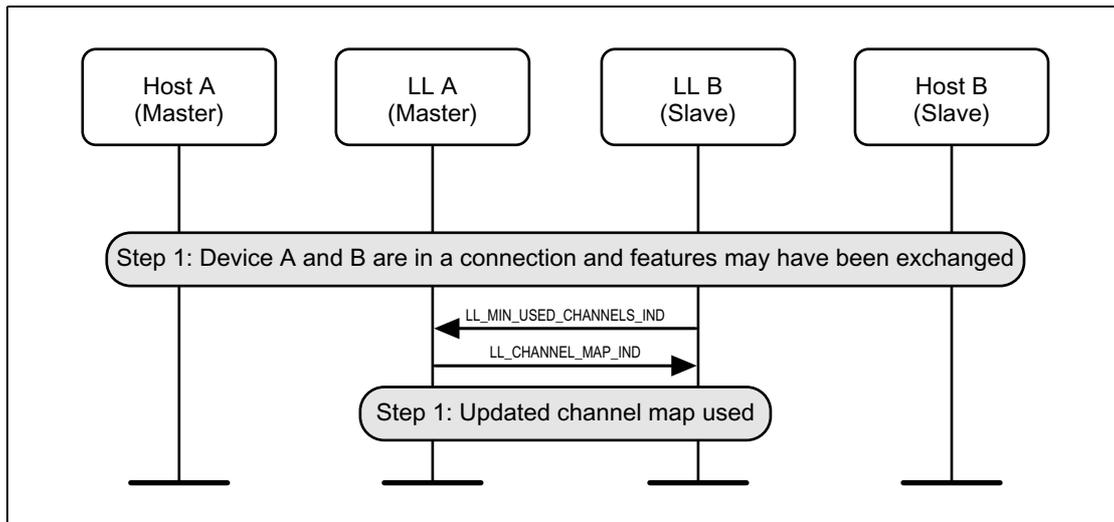
Figure 6.37: Requesting minimum number of used channels
