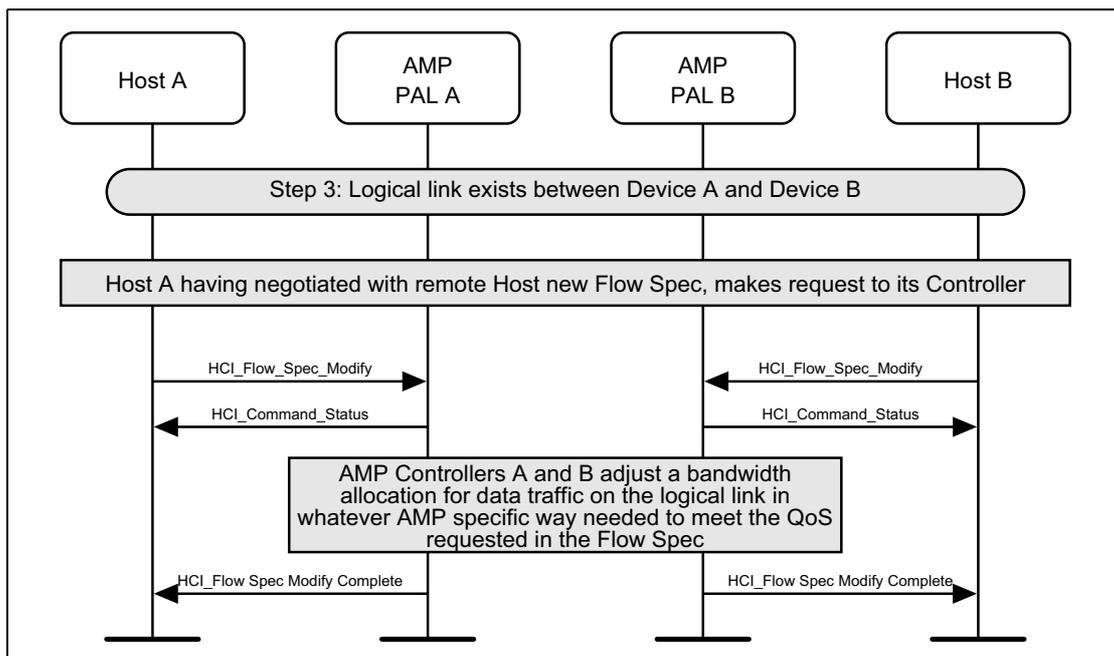
Figure 4.56: Host A modifies Flow\_Spec on an existing logical link
