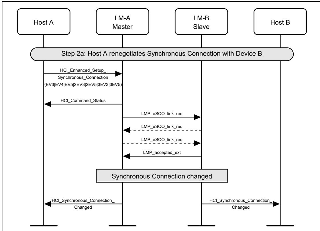
Figure 5.14: Master renegotiates synchronous connection parameter change
