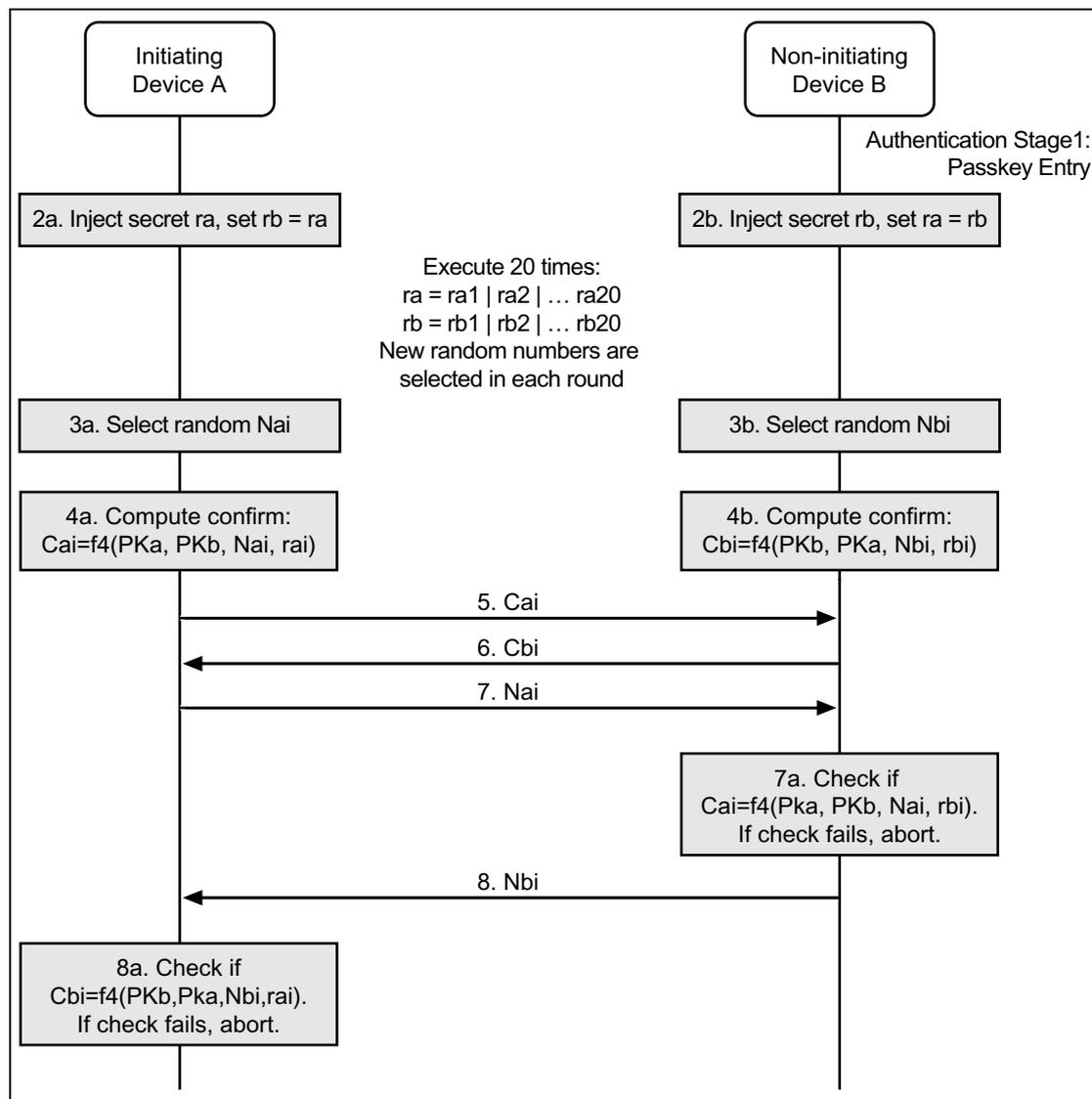
Figure 2.4: Authentication Stage 1: Passkey Entry, LE Secure Connections
