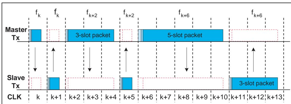
Figure 2.15: Example of the same channel mechanism
