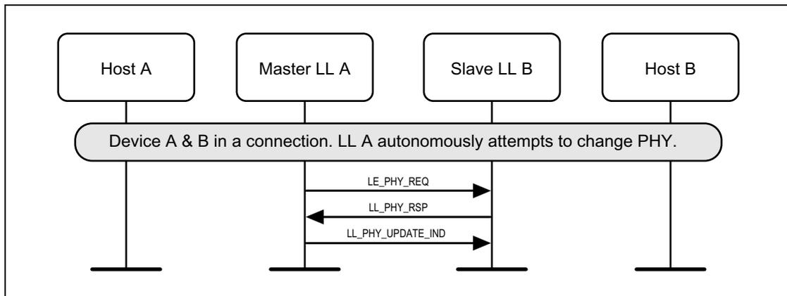
Figure 6.35: Autonomous master-initiated PHY Update procedure – master requests a change of PHY, PHY not changed (either because slave doesn't specify PHYs that the master prefers, or because the master concludes that the current PHYs are still best)
