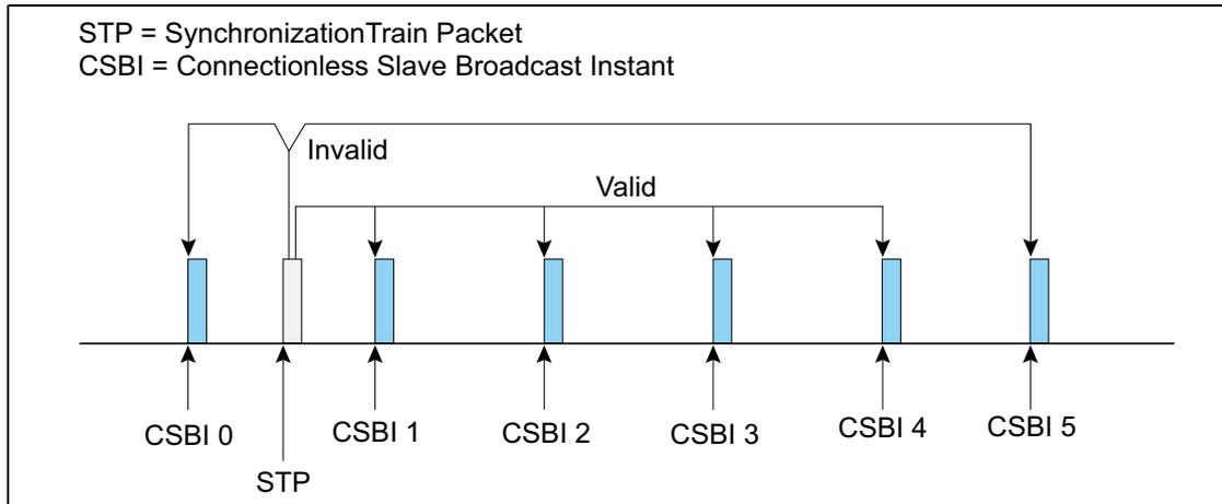
Figure 8.26: Examples of Synchronization Train Pointing to Connectionless Slave Broadcast Instant
