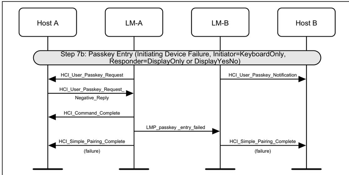
Figure 4.19: Passkey entry failure on initiating side
