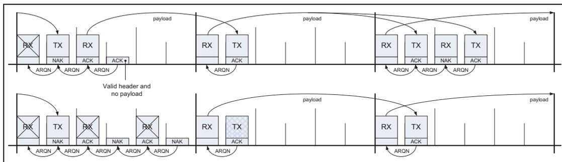
Figure 7.6: Secure Connections eSCO loopback delayed with retransmissions
