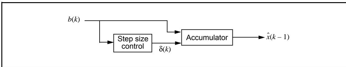
Figure 9.2: Block diagram of CVSD decoder with syllabic companding
