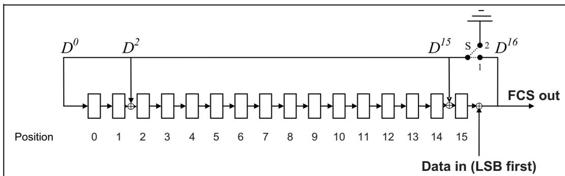
Figure 3.4: The LFSR circuit generating the FCS
