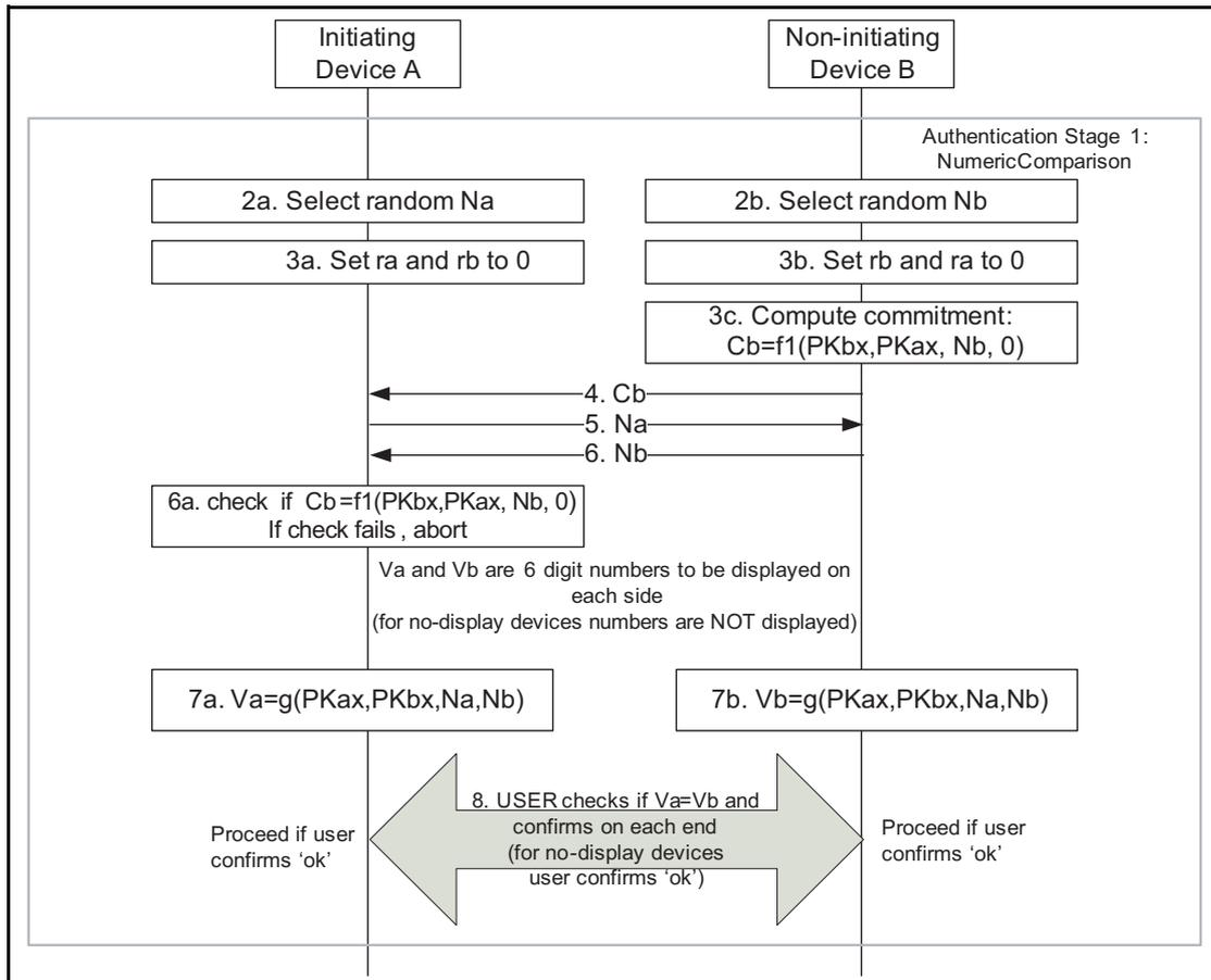
Figure 7.4: Authentication Stage 1: Numeric Comparison Protocol Details
