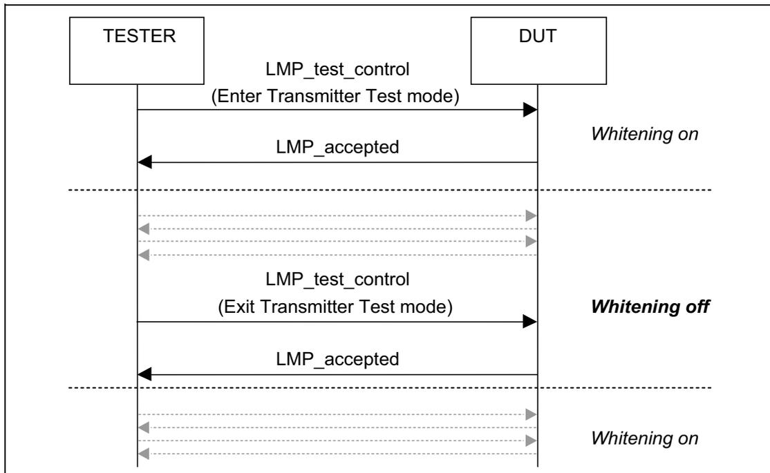
Figure 1.4: Use of whitening in Transmitter mode
