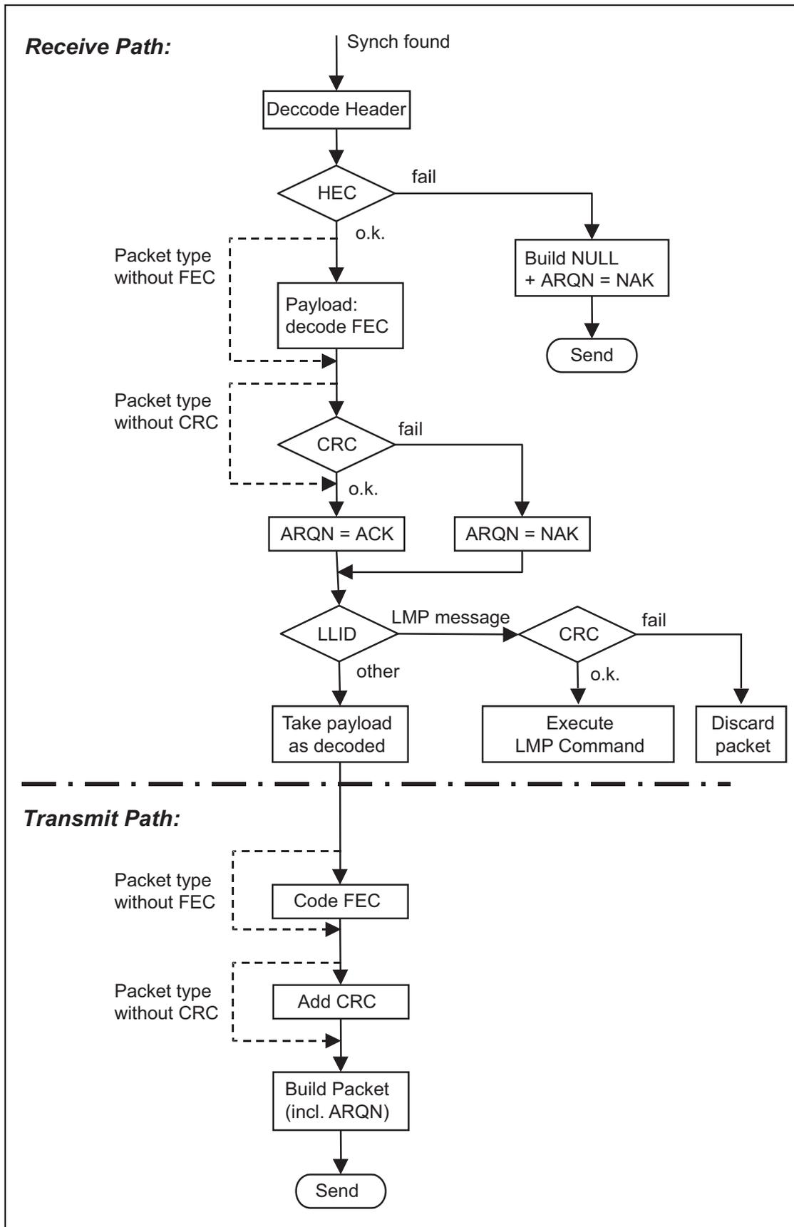
Figure 1.6: DUT Packet Handling in Loop Back Test
