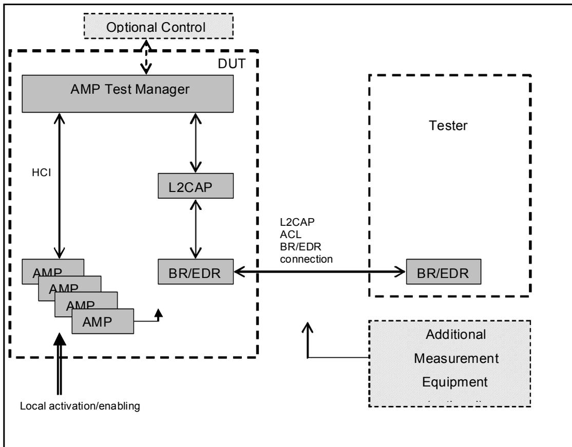
Figure 1.10: Test Architecture
