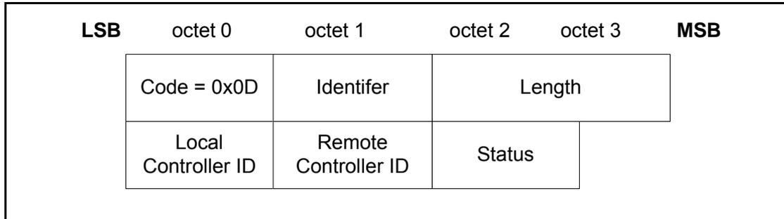
Figure 3.16: AMP Disconnect Physical Link Response Packet
