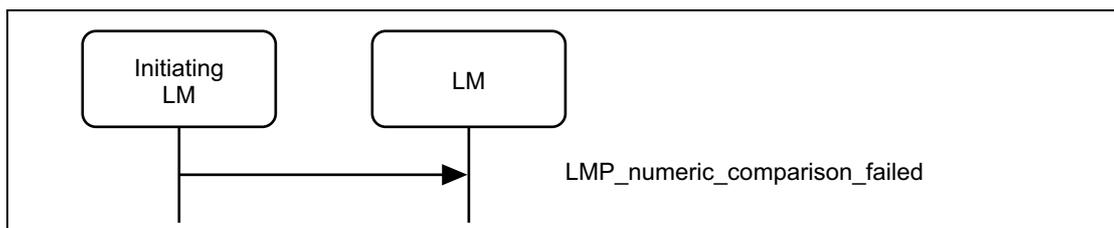
Sequence 62: Authentication stage 1 Numeric Comparison Failure on Initiator Side
