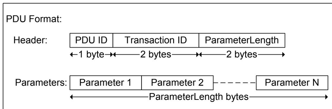
Figure 4.1: Protocol Data Unit Format
