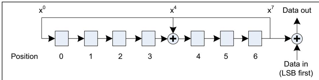
Figure 3.4: The LFSR circuit to generate data whitening
