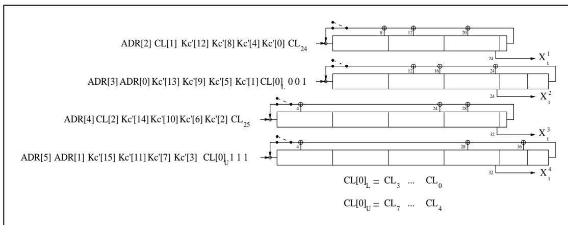
Figure 4.5: Arranging the input to the LFSRs.
