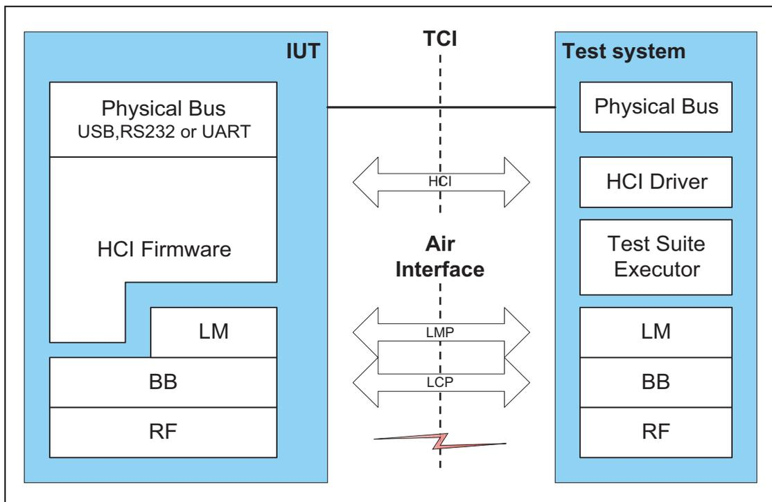
Figure 2.5: General test set-up for HCI qualification
