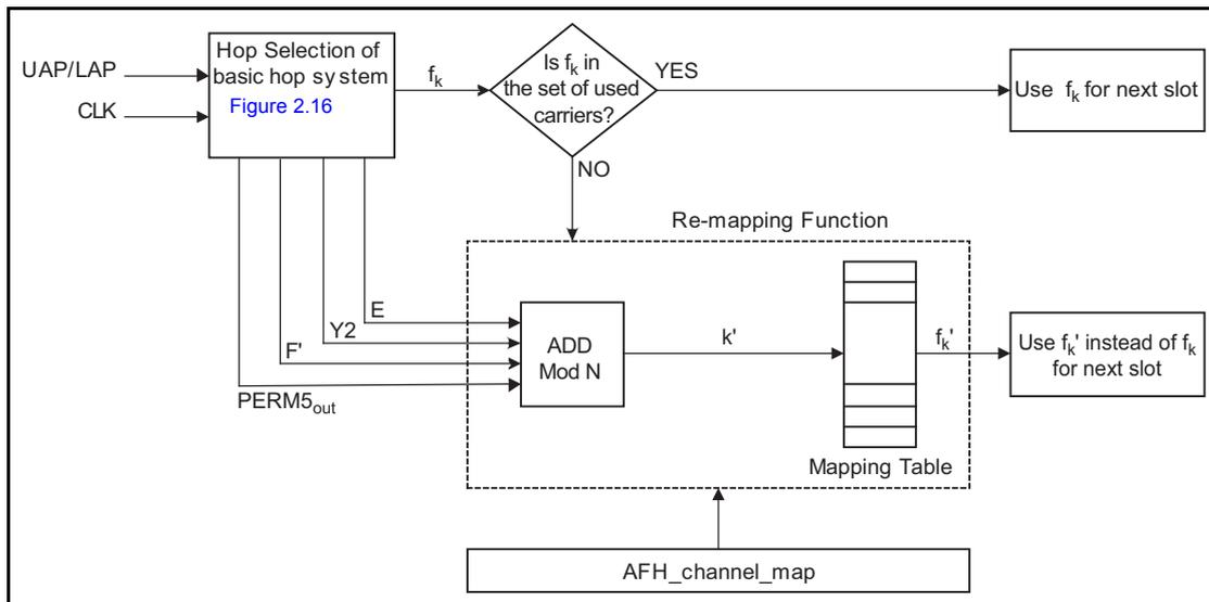
Figure 2.20: Block diagram of adaptive hop selection mechanism
