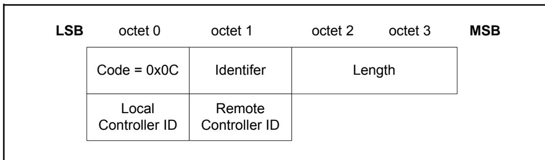
Figure 3.15: AMP Disconnect Physical Link Request Packet
