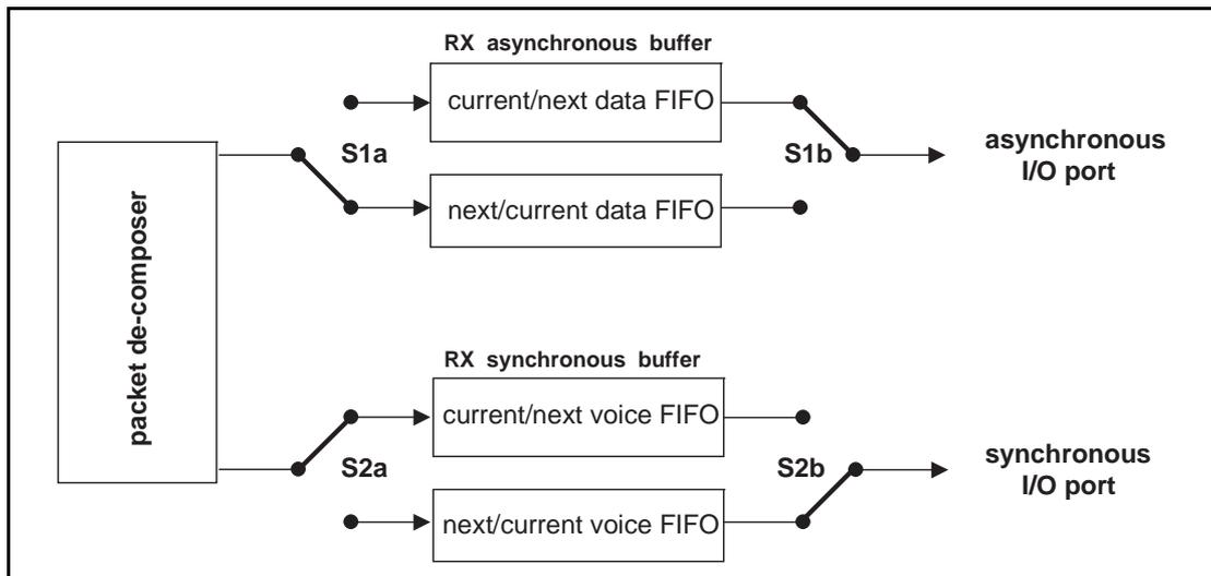
Figure 4.2: Functional diagram of RX buffering
