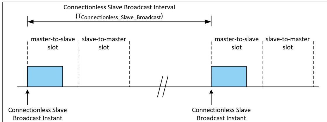
Figure 8.25: Connectionless Slave Broadcast Timing
