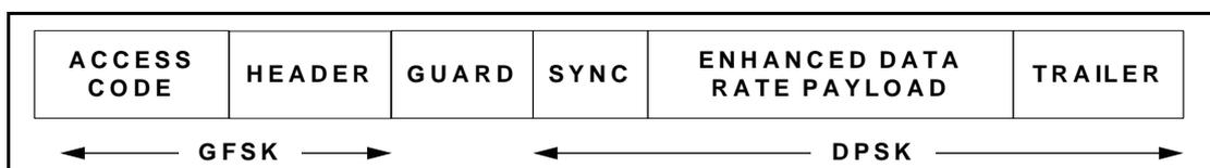
Figure 1.3: Standard Enhanced Data Rate packet format
