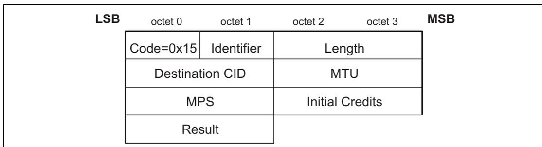
Figure 4.25: LE Credit Based Connection Response Packet
