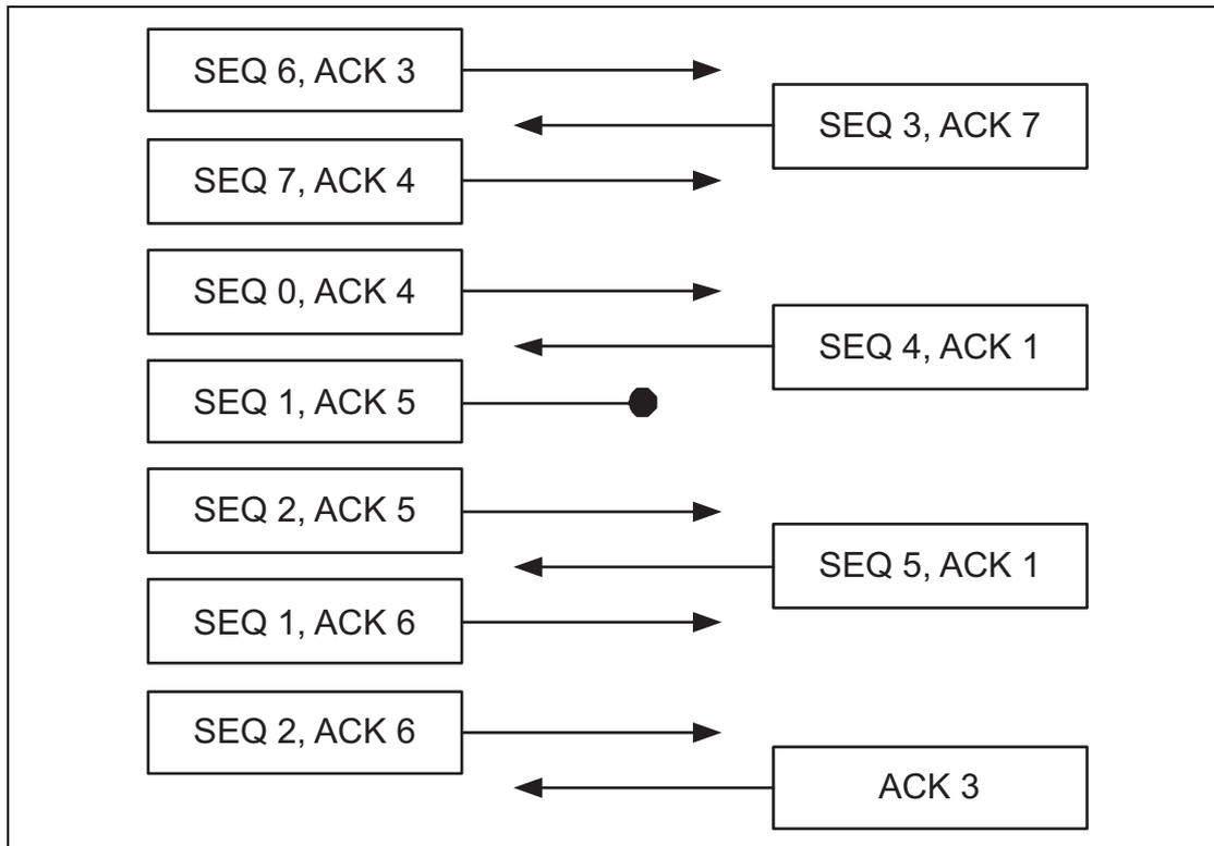
Figure 6.1: Message Diagram Showing Transmission of Reliable Packets
