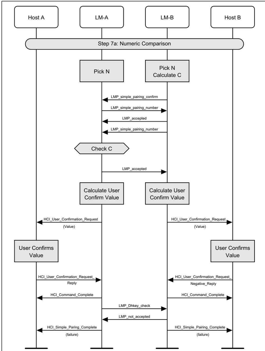
Figure 4.16: Numeric comparison failure on responding side
