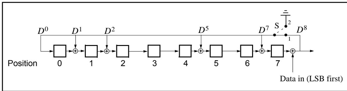
Figure 7.3: The LFSR circuit generating the HEC
