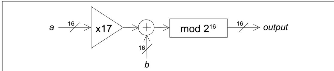
Figure 4.35: Multiply, Add, and Modulo block operation
