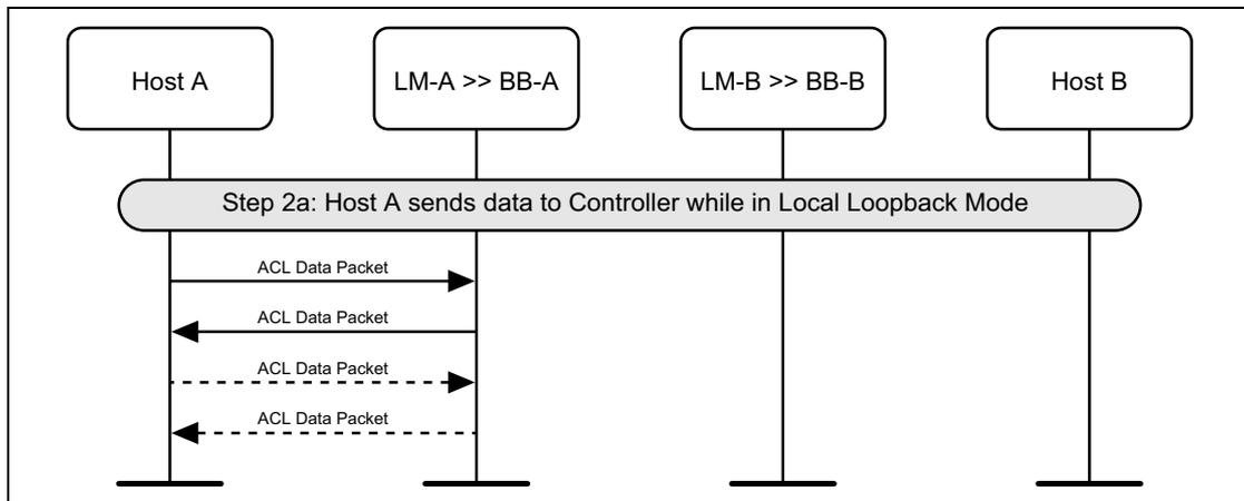
Figure 8.2: Looping back data in local loopback mode
