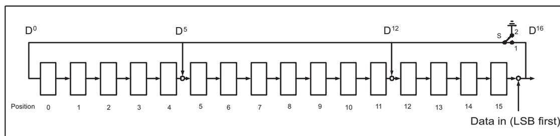
Figure 5.1: The LFSR Circuit Generating the CRC
