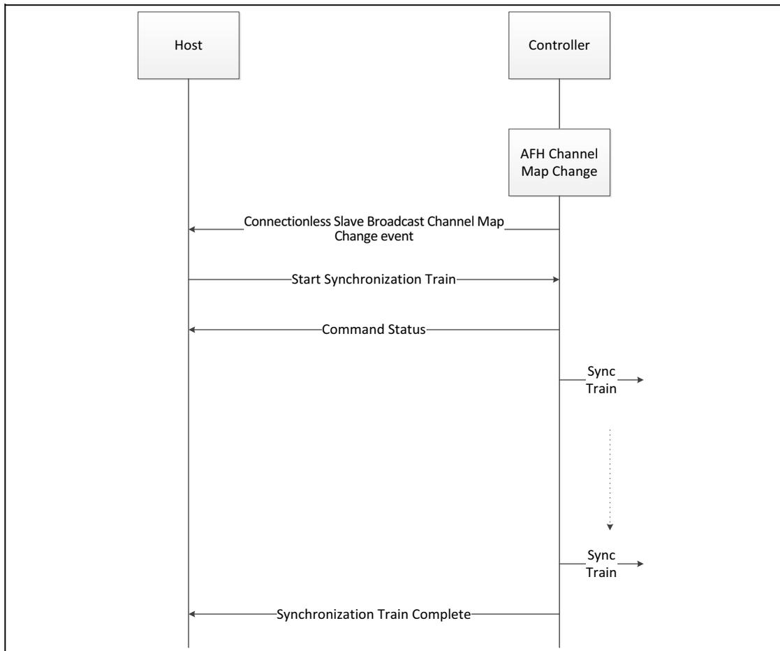
Figure C.2: AFH Map Change – Connectionless Slave Broadcast master
