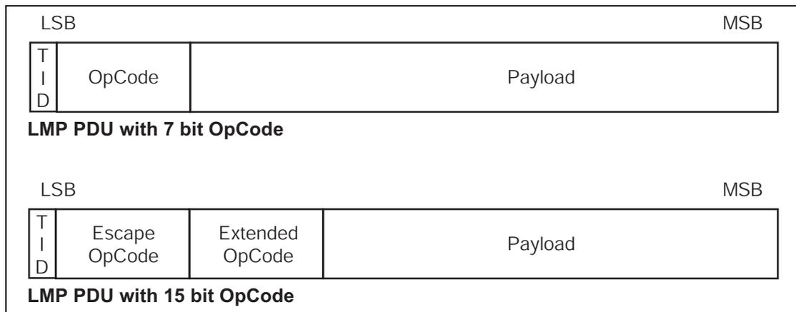
Figure 2.2: Payload body when LMP PDUs are sent
