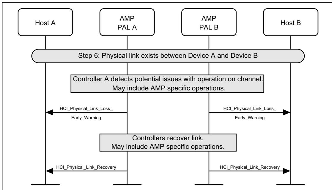
Figure 4.53: Controller reports link loss to its Host
