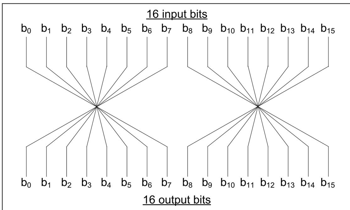
Figure 4.34: Permutation operation
