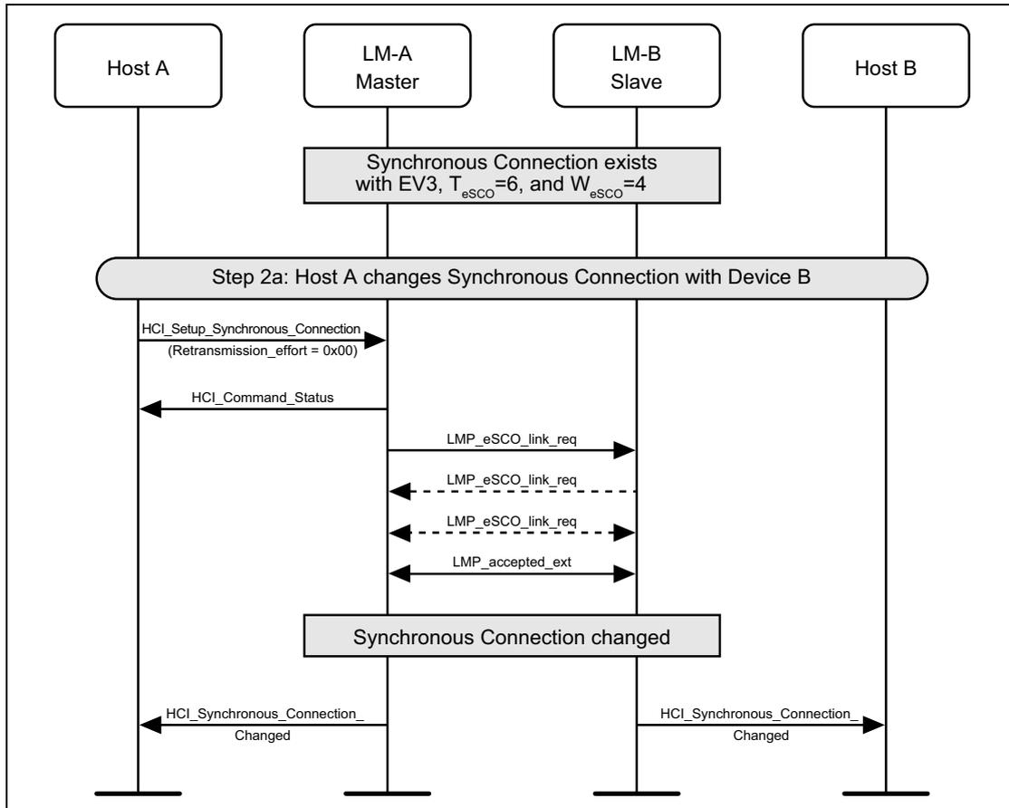
Figure 5.6: Master renegotiates eSCO connection
