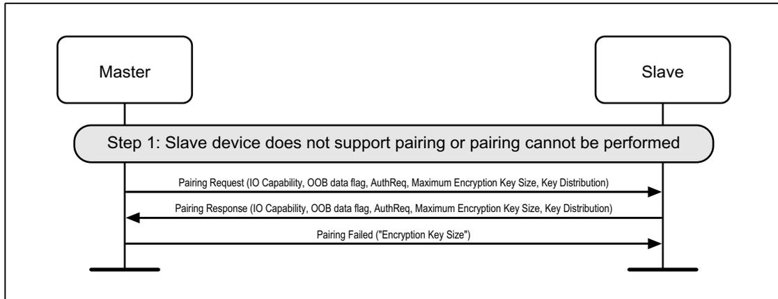
Figure C.27: Master rejects pairing because of key size
