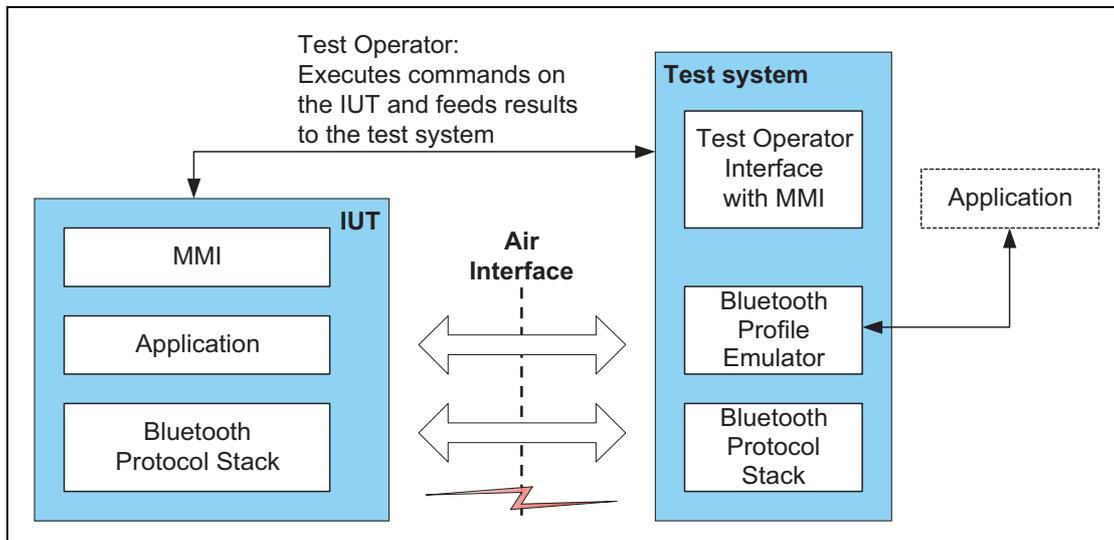
Figure 2.2: General test set-up for profile qualification
