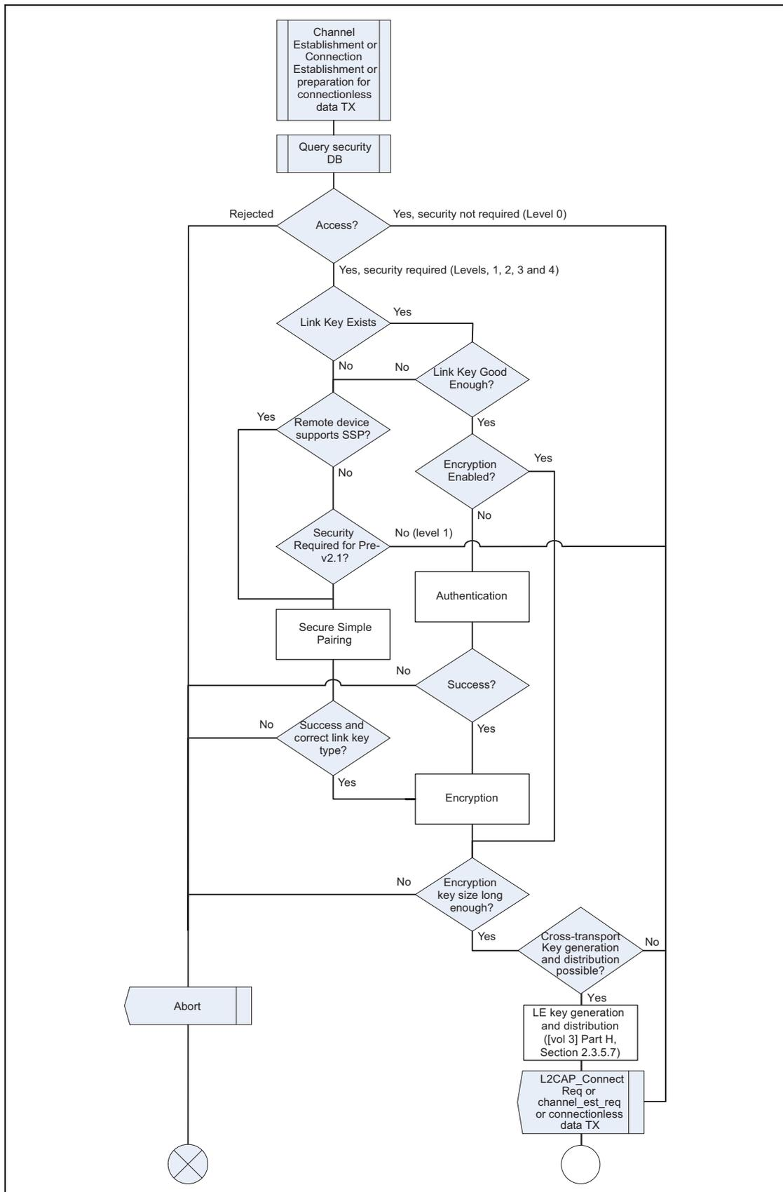
Figure 5.4: Channel establishment using security mode 4 for initiating side
