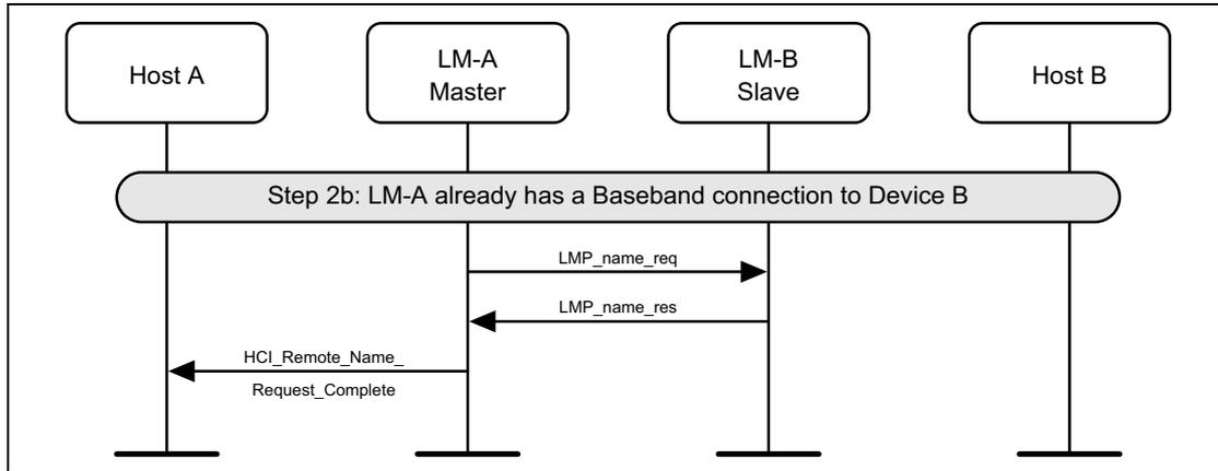
Figure 2.3: Remote name request with baseband connection
