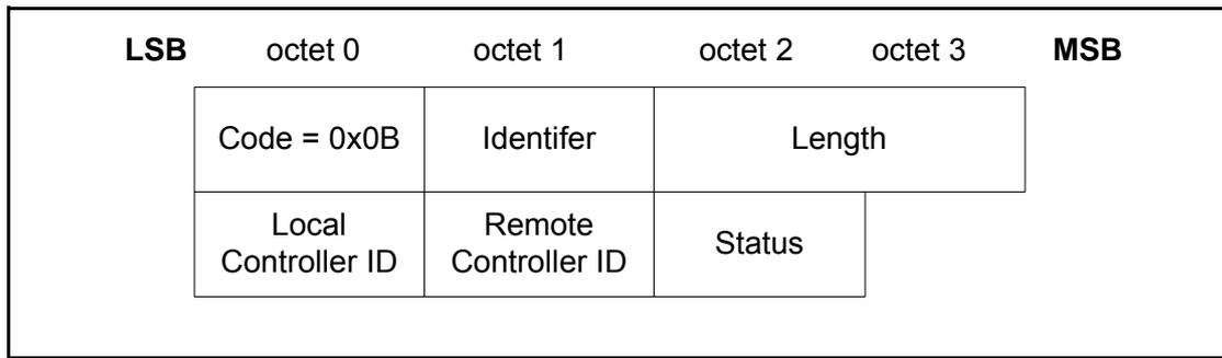
Figure 3.14: AMP Create Physical Link Response Packet
