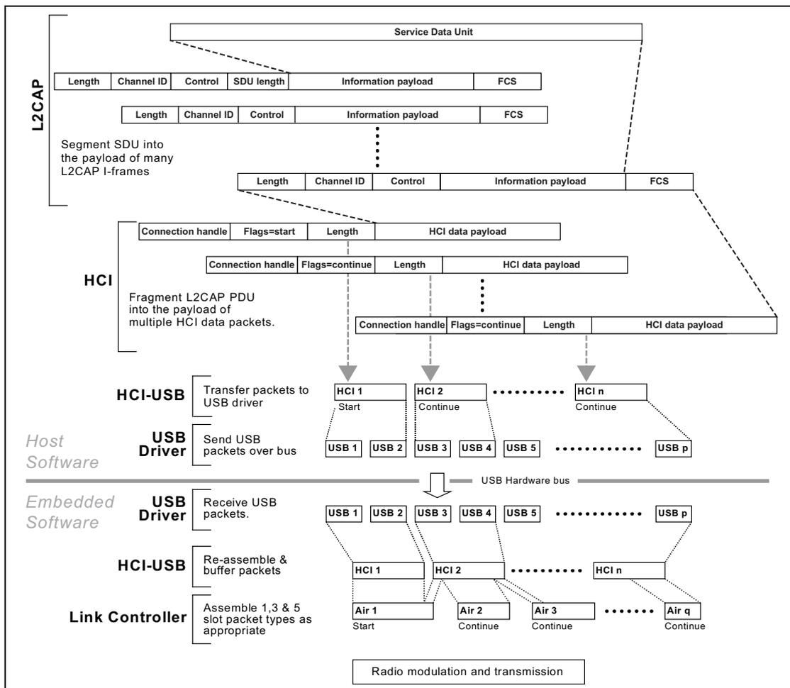
Figure 7.4: Example of segmentation and fragment processes in a device with a BR/EDR Controller and USB HCI Transport<sup>1</sup>
