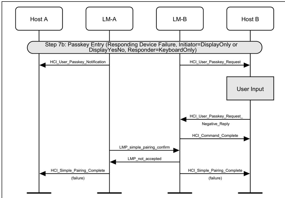
Figure 4.18: Passkey entry failure on responding side
