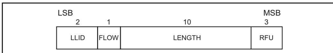
Figure 6.13: Payload header format for multi-slot ACL packets and all EDR ACL packets
