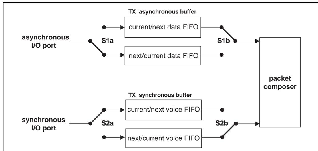
Figure 4.1: Functional diagram of TX buffering
