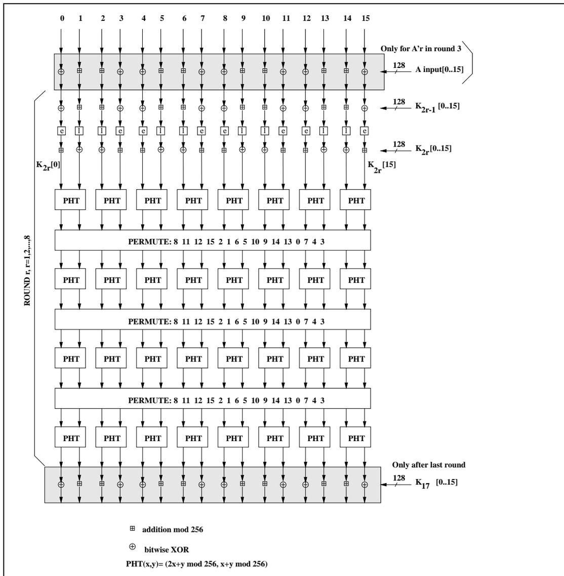
Figure 6.2: One round in A<sub>r</sub> and A'<sub>r</sub>
