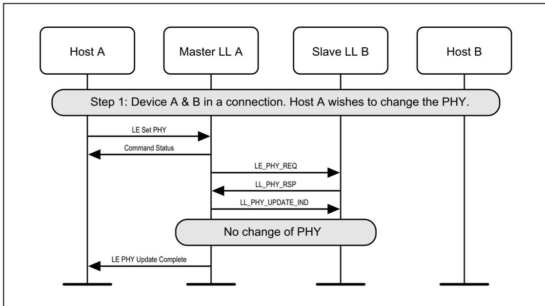
Figure 6.29: Master initiated PHY Update procedure, PHY not changed (either because slave doesn't specify PHYs that the master prefers, or because the master concludes that the current PHYs are still best)
