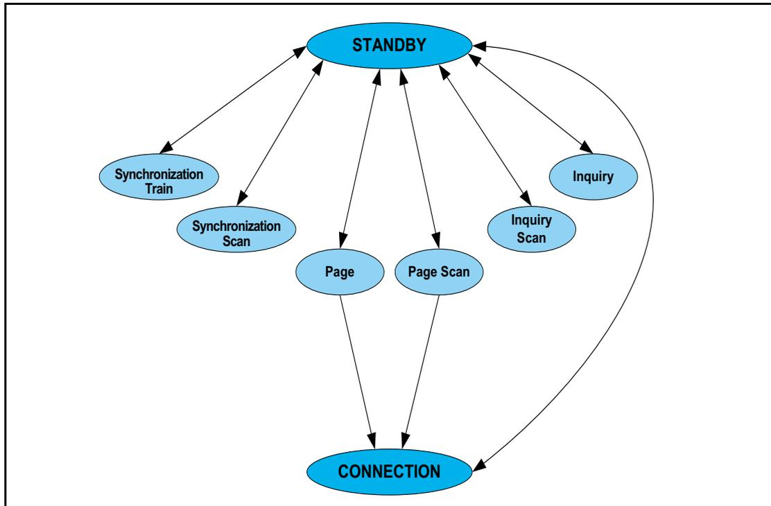
Figure 8.1: State diagram of Link Controller
