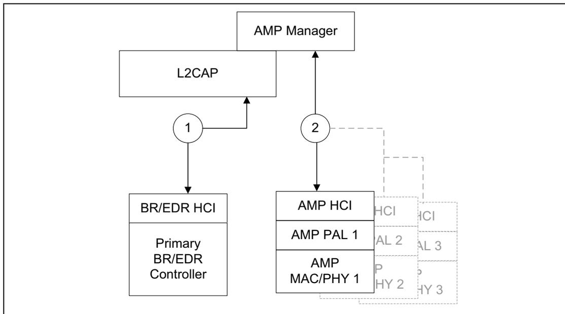
Figure 2.1: Overview of the Lower Software Layers
