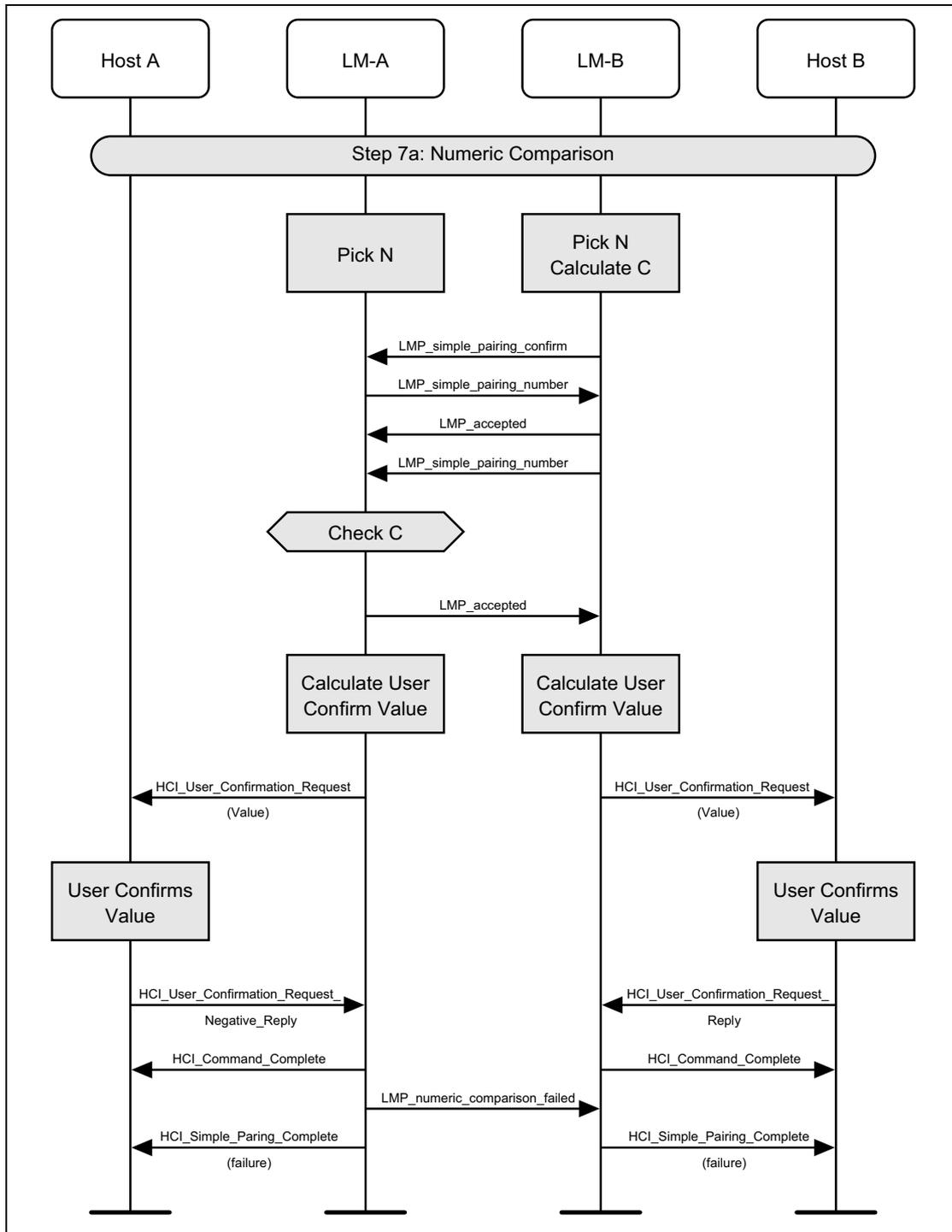
Figure 4.15: Numeric comparison authentication (failure on initiating side)
