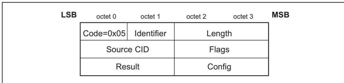
Figure 4.8: Configuration Response Packet
