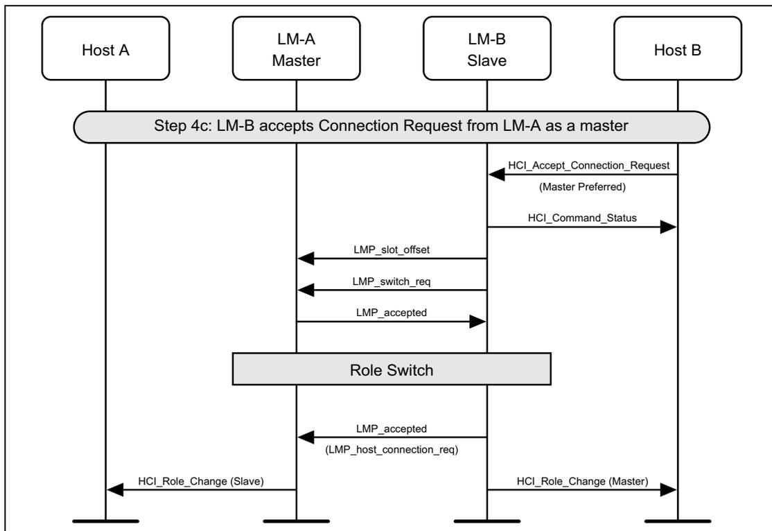
Figure 3.7: Device B accepts connection requests as master
