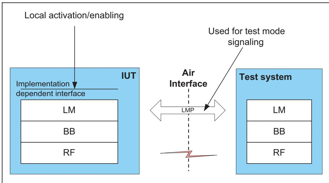
Figure 2.1: General test set-up for RF qualification
