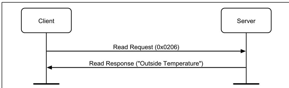
Figure 4.19: Read Characteristic Descriptors example
