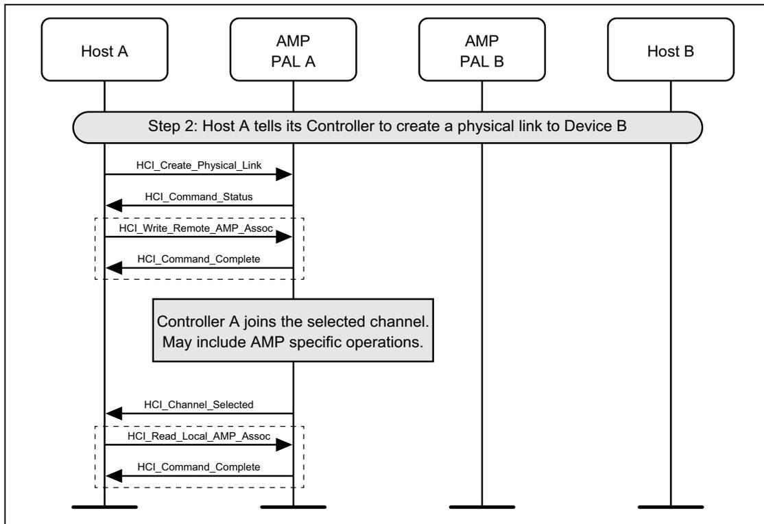
Figure 4.49: Host A tells its Controller to create the physical link
