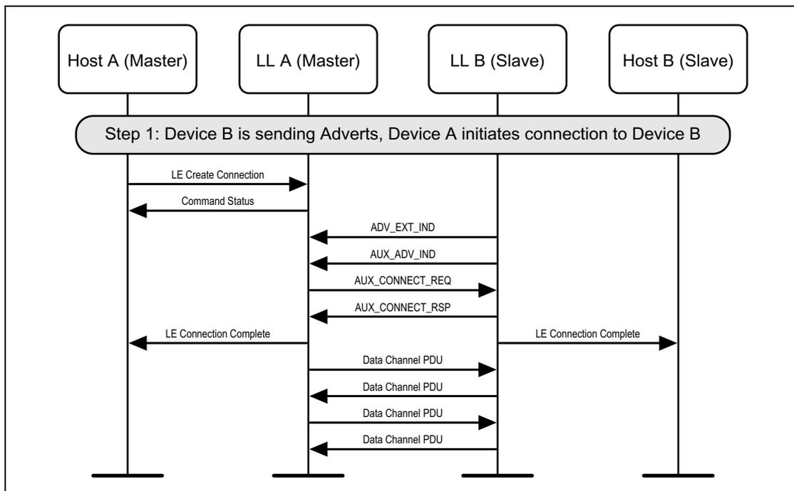
Figure 5.6: Initiating a connection on the secondary advertising channel
