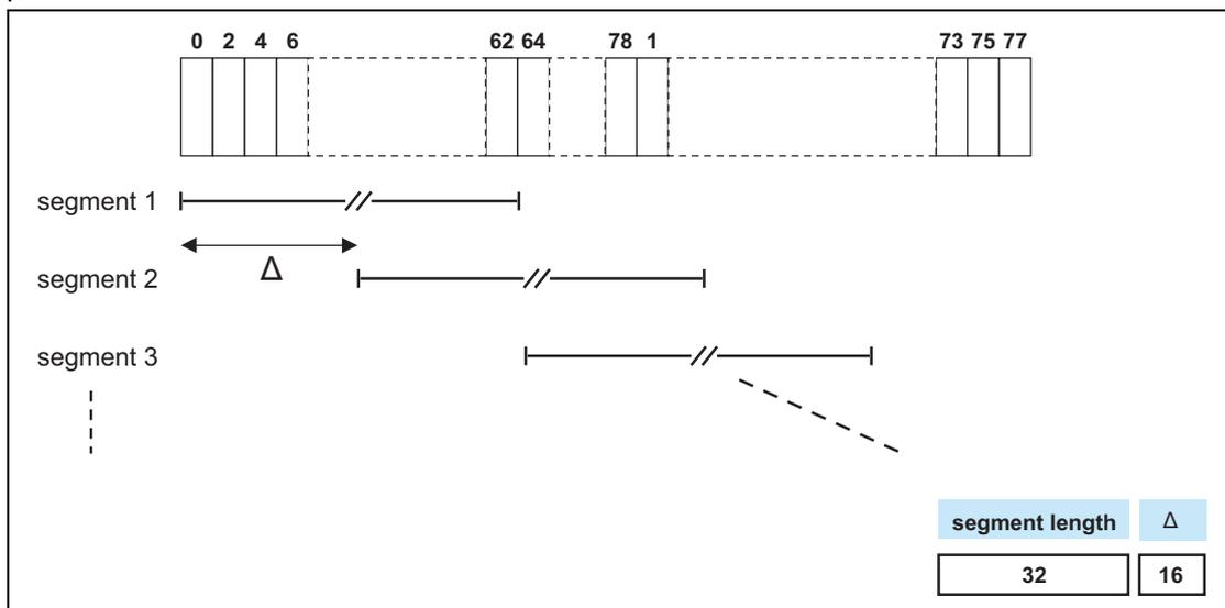
Figure 2.13: Hop selection scheme in CONNECTION state
