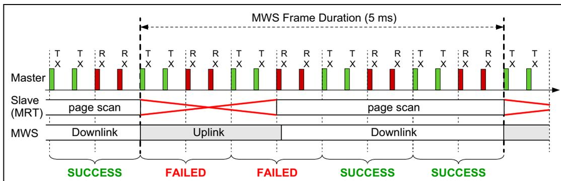
Figure 7.5: Bluetooth radio can suffer inquiry scan/page scan failures
