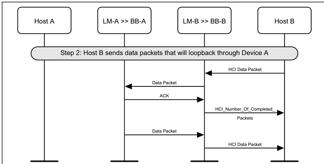
Figure 8.6: Looping back data in remote loopback mode
