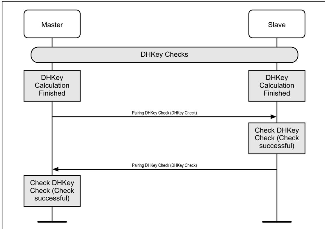
Figure C.23: Pairing Phase 2, Authentication Stage 2, DHKey checks
