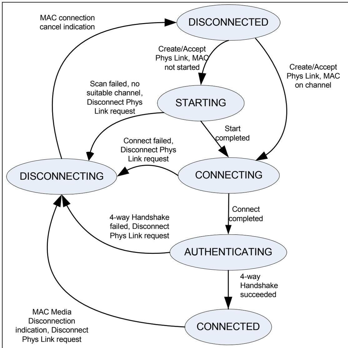
Figure 3.1: Physical Link finite state machine diagram
