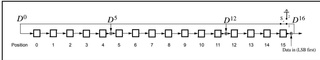
Figure 7.6: The LFSR circuit generating the CRC
