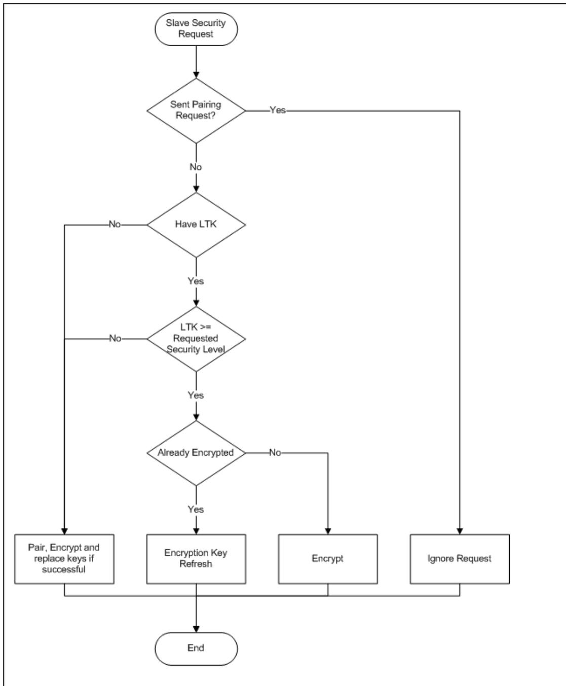
Figure 2.7: Master actions after receiving Security Request
