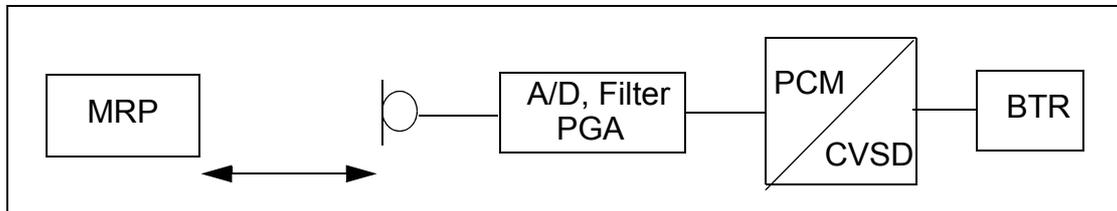
Figure A.1: SLR measurement set-up
