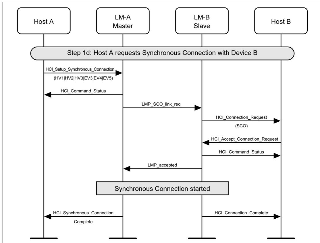
Figure 5.4: Master requests synchronous connection with legacy slave
