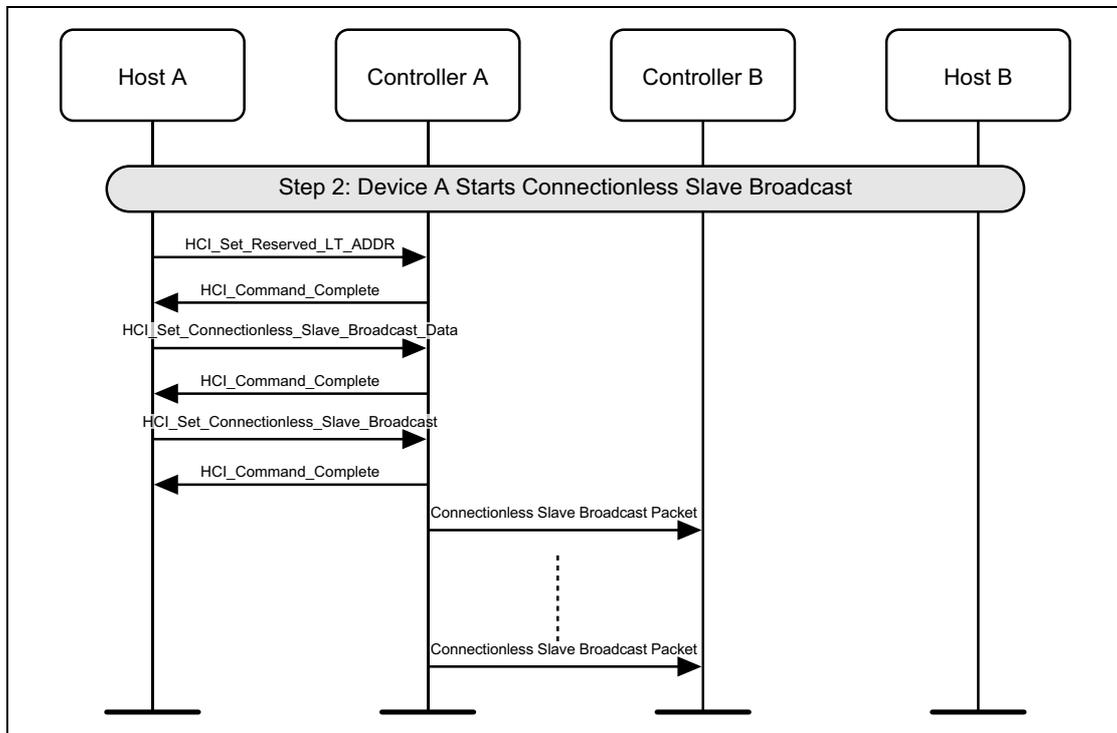
Figure 9.2: Connectionless slave broadcast transmitter start
