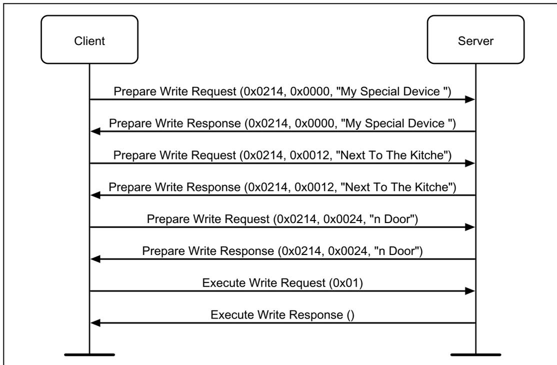
Figure 4.22: Write Long Characteristic Descriptors example
