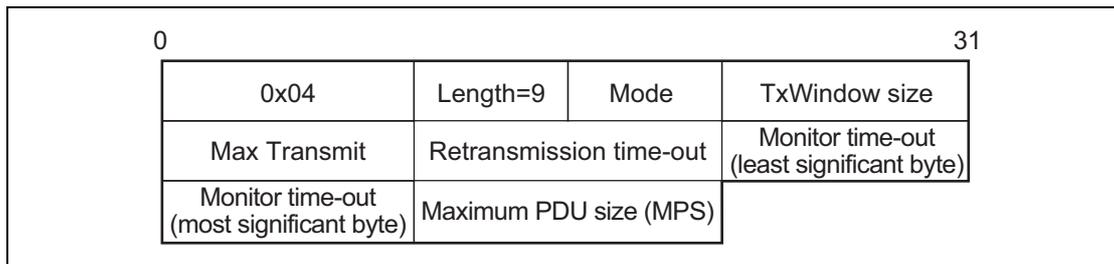
Figure 5.5: Retransmission and Flow Control option format
