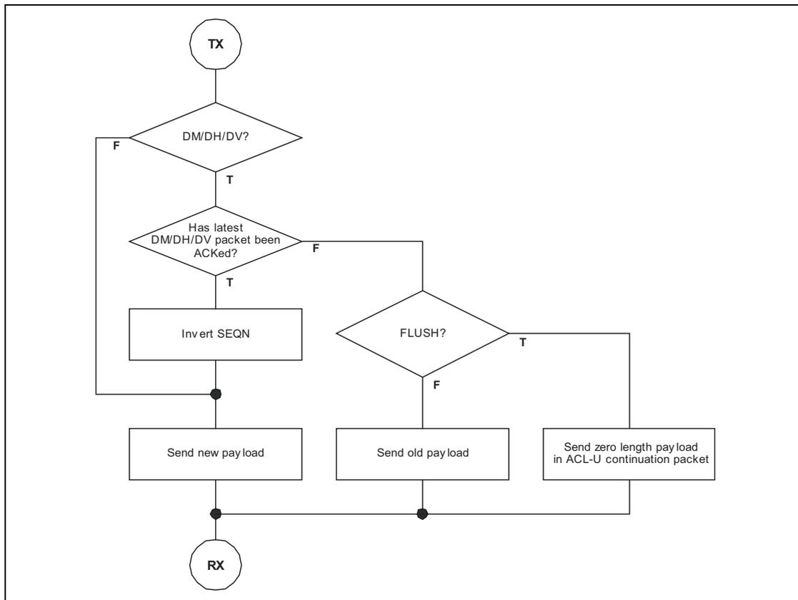
Figure 7.15: Transmit filtering for packets with CRC
