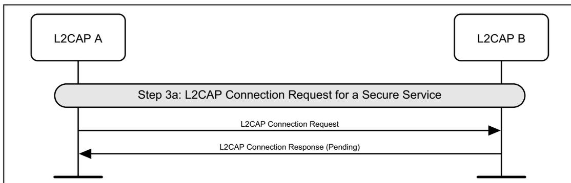
Figure 4.9: *L2CAP connection request for a secure service*
