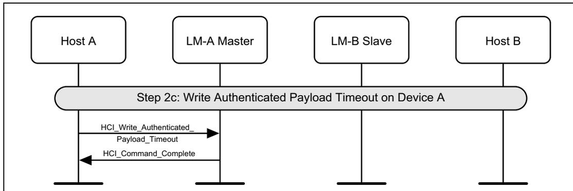
Figure 4.8: Set *Authenticated\_Payload\_Timeout*
