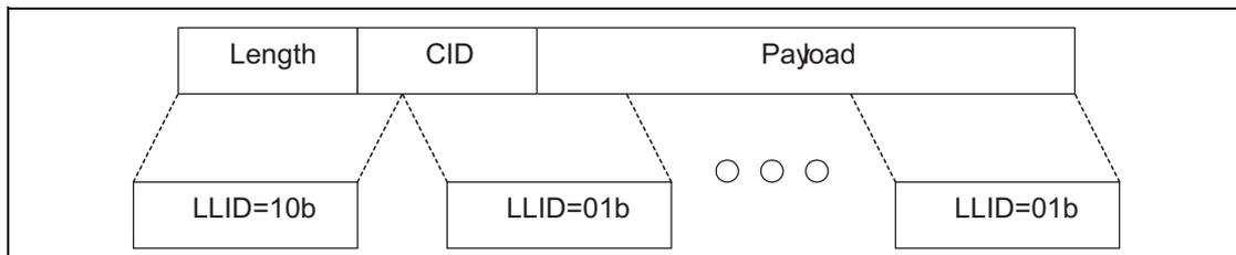
Figure 7.1: L2CAP fragmentation in a BR/EDR Controller
