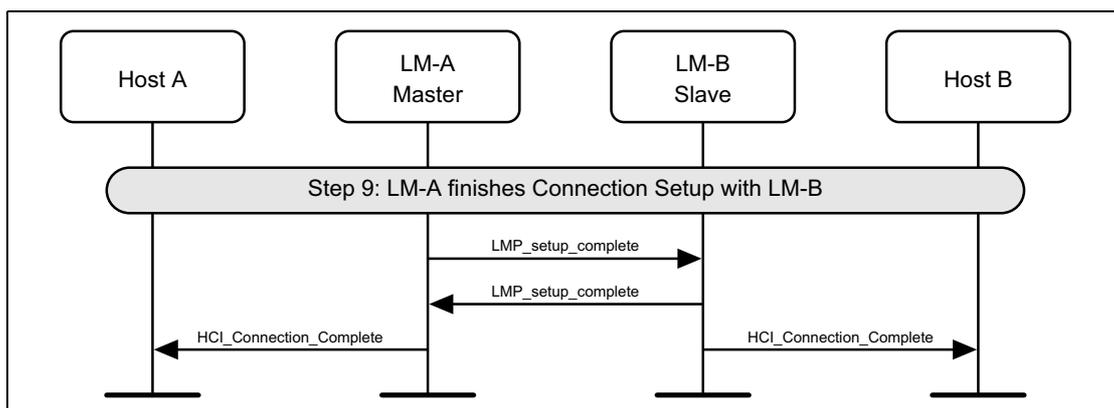
Figure 3.13: LM-A and LM-B finishes connection setup
