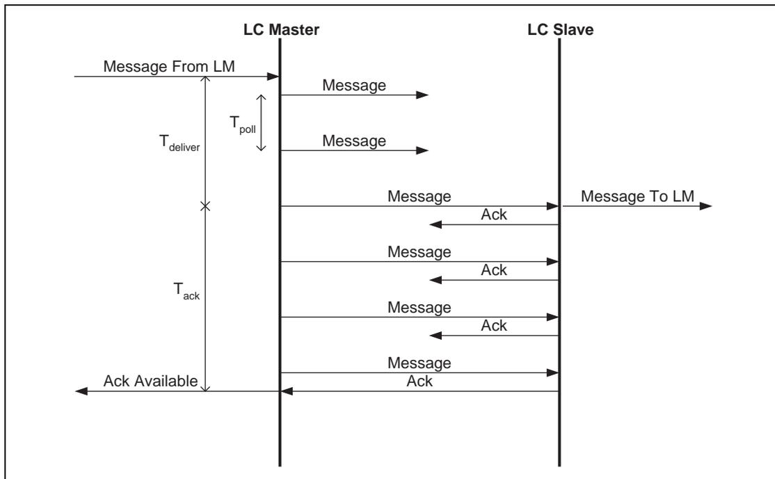
Figure 2.1: Transmission of a message from master to slave<sup>1</sup>
