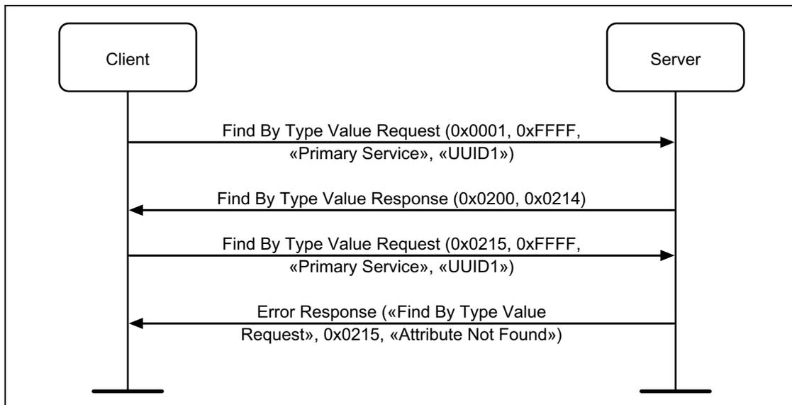
Figure 4.3: Discover Primary Service by Service UUID example
