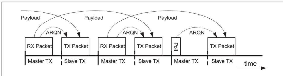
Figure 1.9: Payload & ARQN handling in delayed loopback - end.
