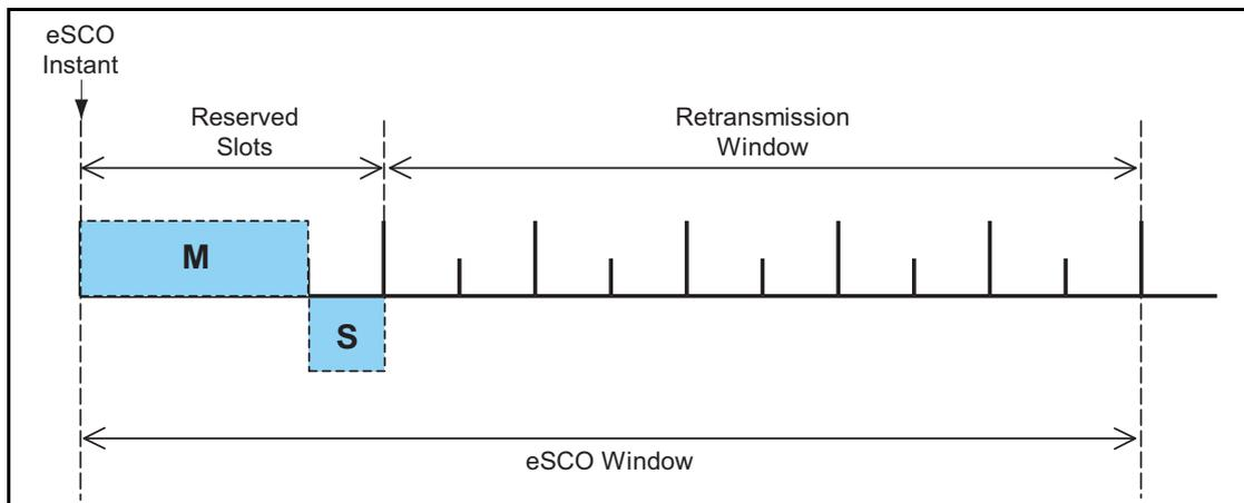
Figure 8.10: eSCO Window Details for Asymmetric Traffic
