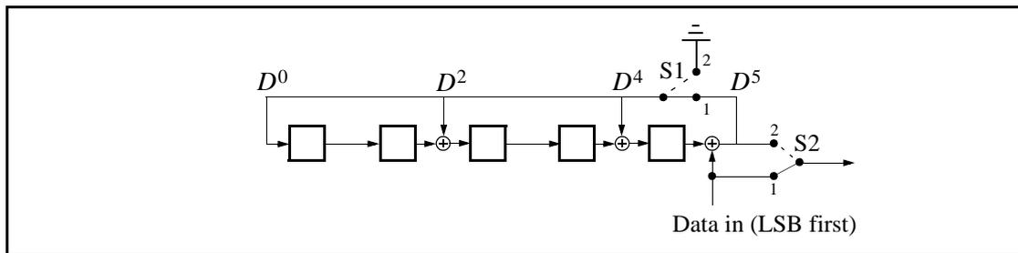
Figure 7.11: LFSR generating the (15,10) shortened Hamming code
