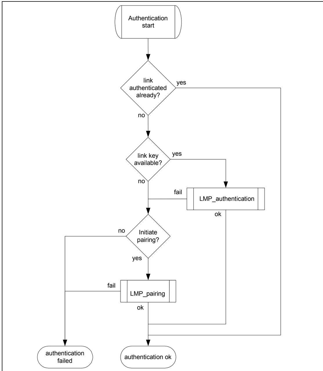
Figure 5.1: Definition of the generic authentication procedure
