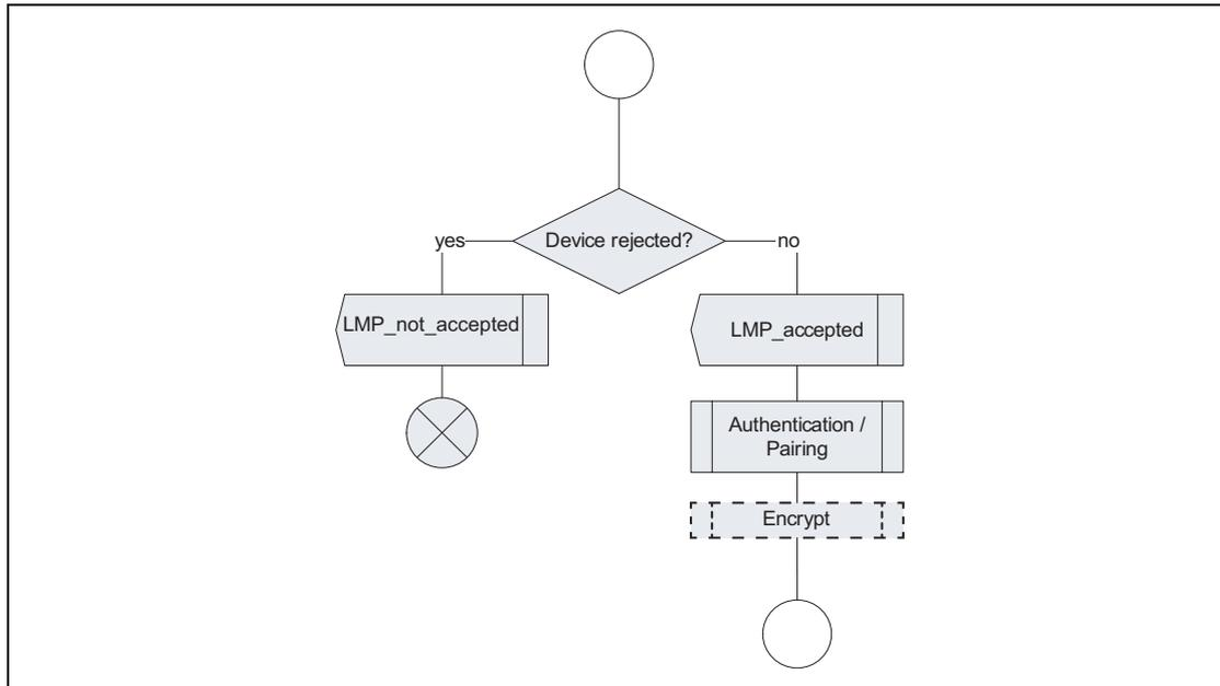
Figure 5.3: Security mode 3 with a legacy remote device
