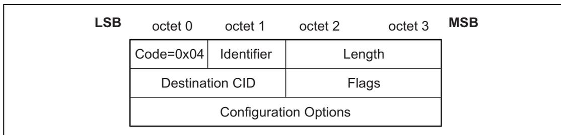
Figure 4.6: Configuration Request Packet
