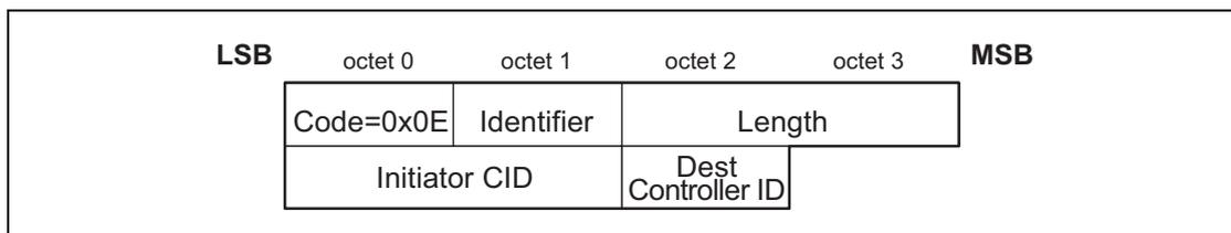
Figure 4.18: Move Channel Request Packet
