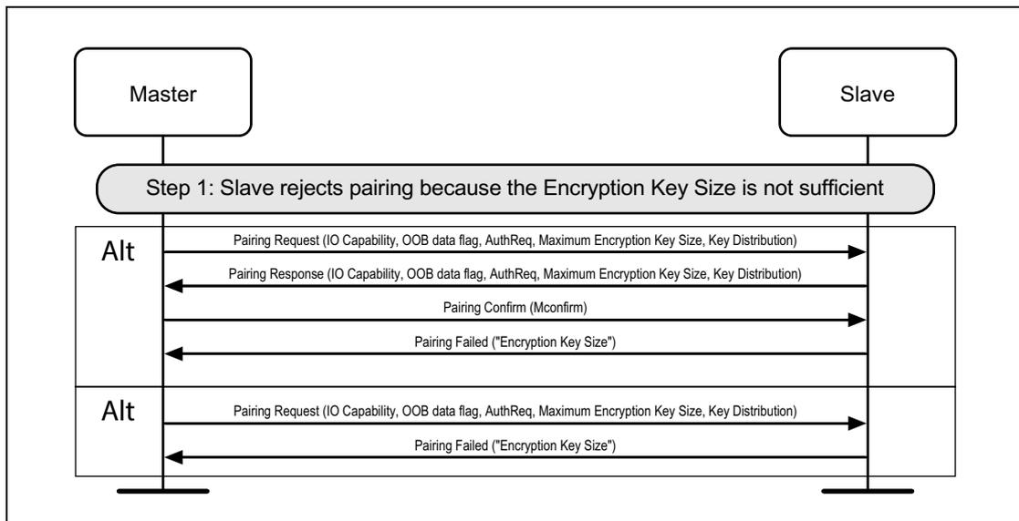
Figure C.28: Slave rejects pairing because of key size
