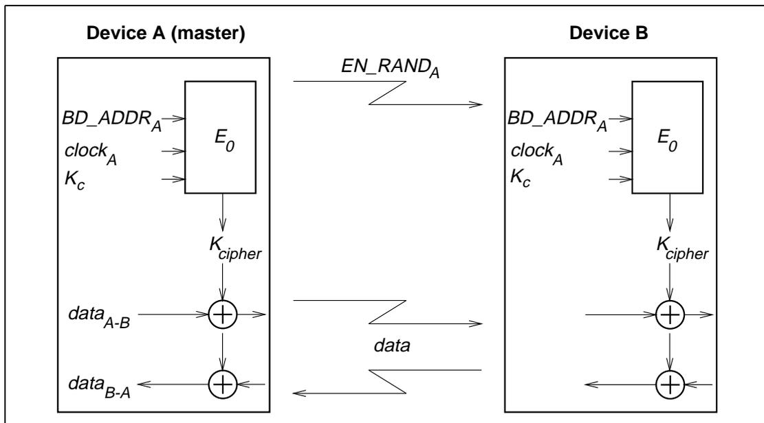
Figure 4.2: Functional description of the encryption procedure
