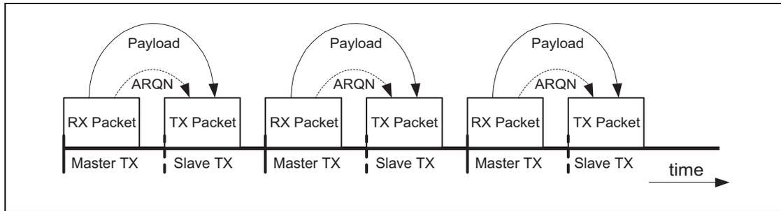
Figure 1.7: Payload & ARQN handling in normal loopback.
