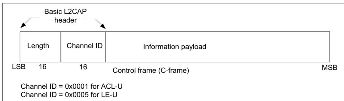
Figure 4.1: L2CAP PDU format on a signaling channel
