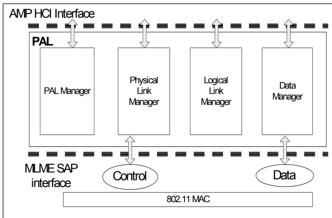
Figure 1.1: Internal structure of the 802.11 PAL
