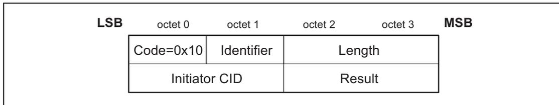
Figure 4.20: Move Channel Confirmation Packet
