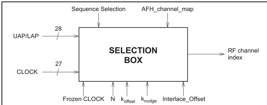
Figure 2.12: General block diagram of hop selection scheme
