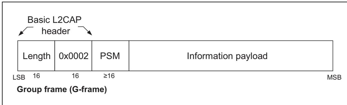
Figure 3.2: L2CAP PDU format on the Connectionless channel
