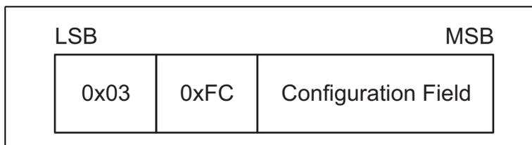
Figure 8.4: Configuration Message Format
