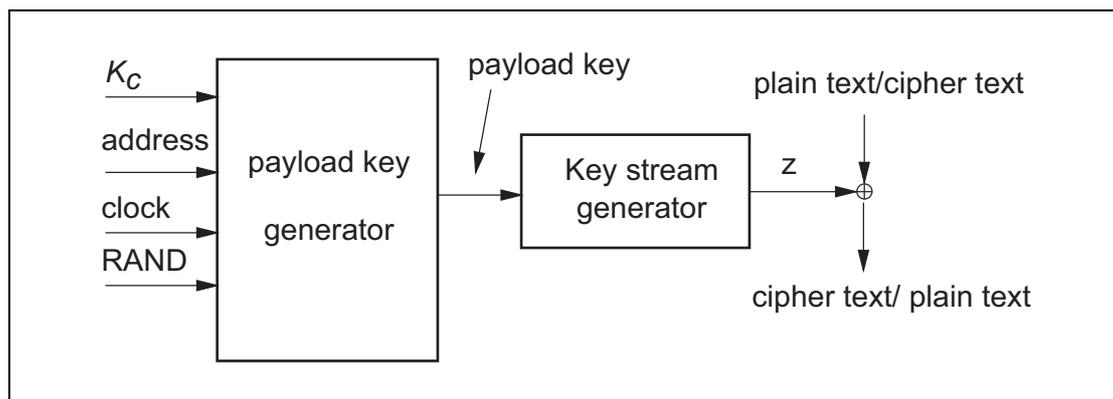
Figure 4.1: Stream ciphering for Bluetooth with  $E_0$ .
