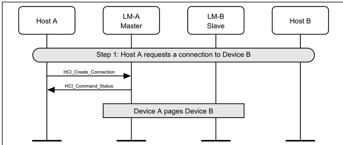
Figure 3.2: Host A requests connection with device B
