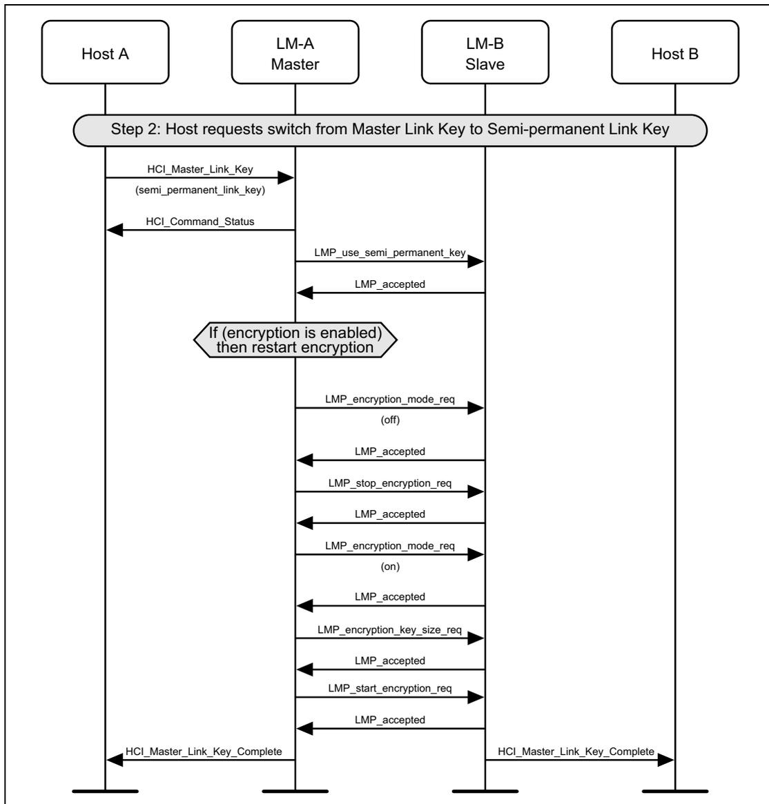
Figure 4.35: Change to semi permanent link key
