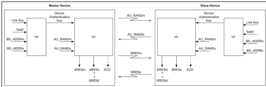
Figure 5.3: Challenge and response for secure authentication.
