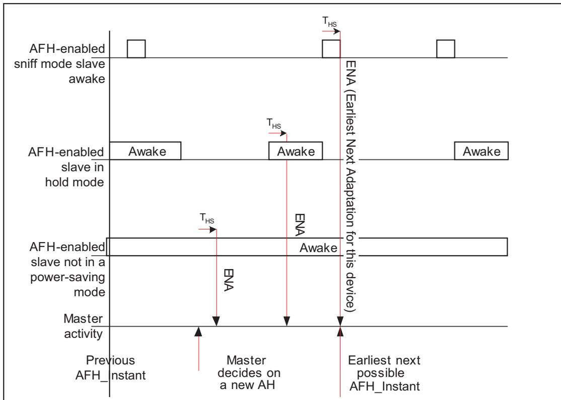
Figure C.1: Timing constraint on AFH\_Instance with slaves in hold and sniff
