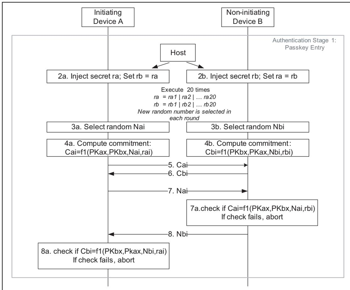
Figure 7.6: Authentication Stage 1: Passkey Entry Details
