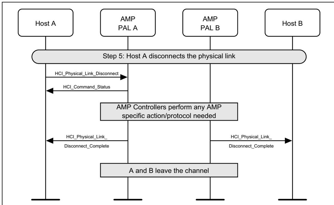
Figure 4.52: Host A disconnects the physical link
