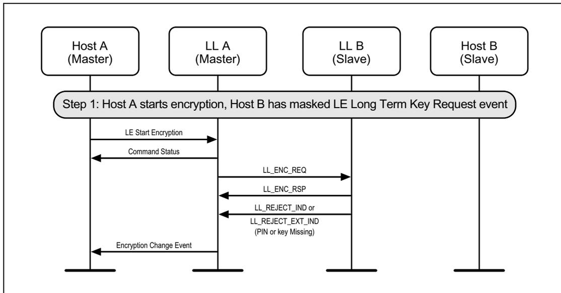
Figure 6.10: Start encryption with slave masking out event
