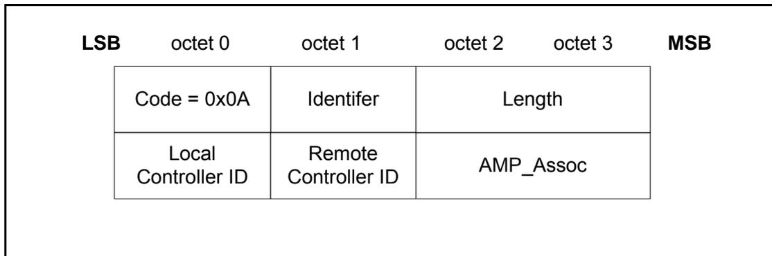
Figure 3.13: AMP Create Physical Link Request Packet
