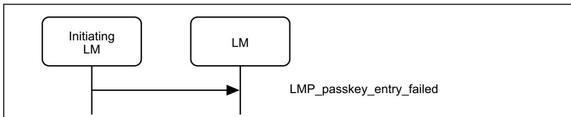
Sequence 67: Authentication stage 1 Passkey Entry Failure on Initiator Side
