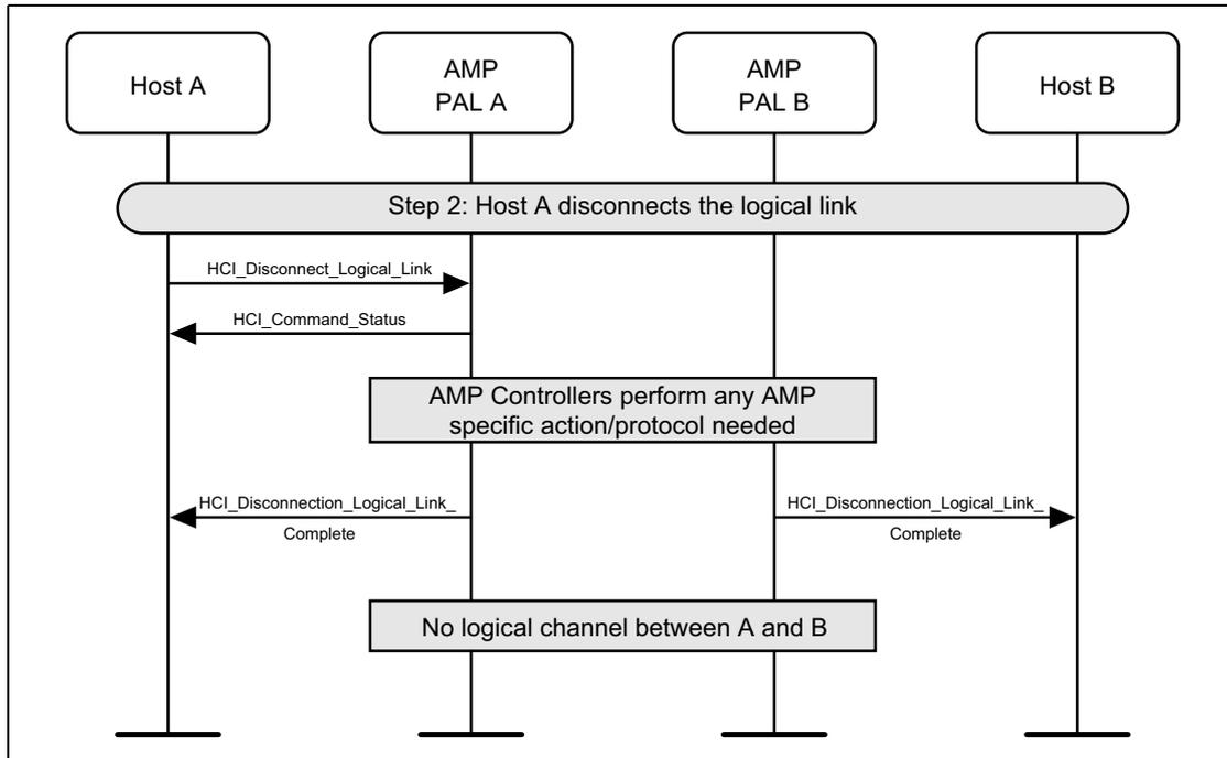
Figure 4.55: Host A disconnects the logical link
