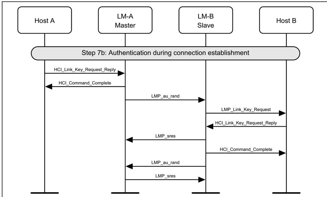
Figure 3.11: Authentication during connection setup
