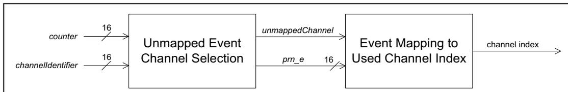
Figure 4.33: General block diagram of Channel Selection Algorithm #2
