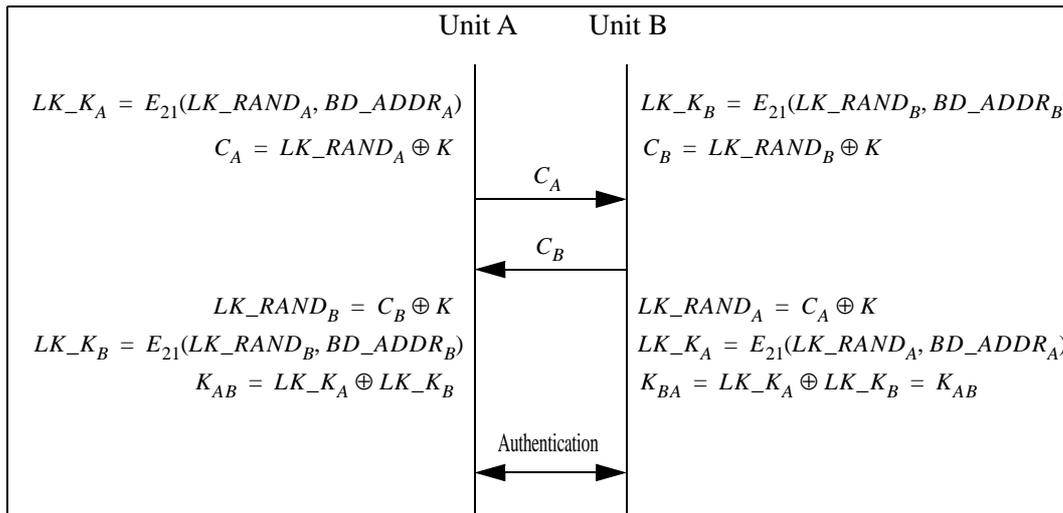
Figure 3.2: Generating a combination key. The old link key ( $K$ ) is discarded after the exchange of a new combination key has succeeded
