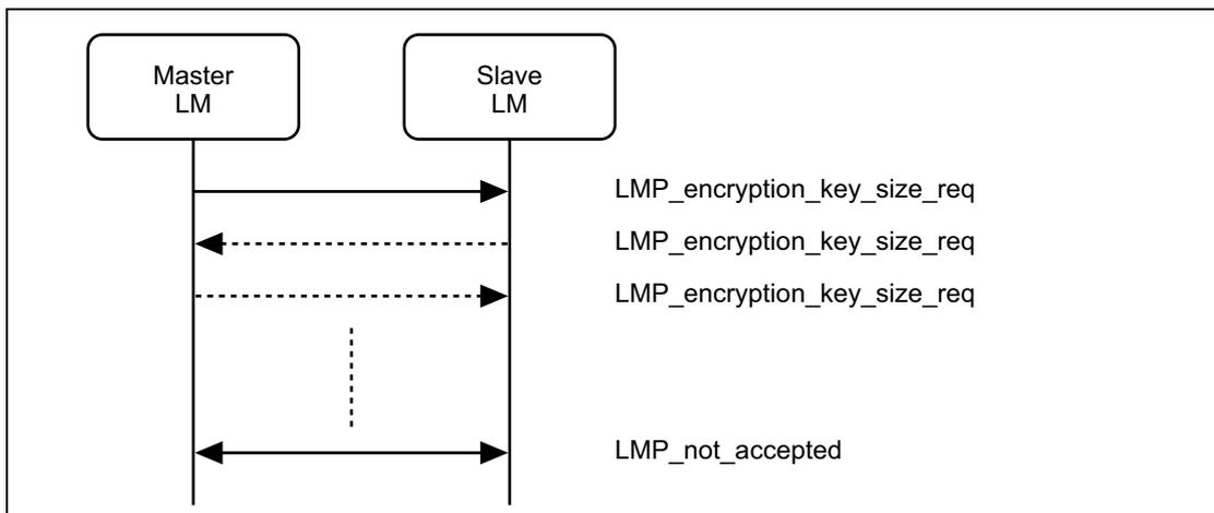
Sequence 46: Encryption key size negotiation failed
