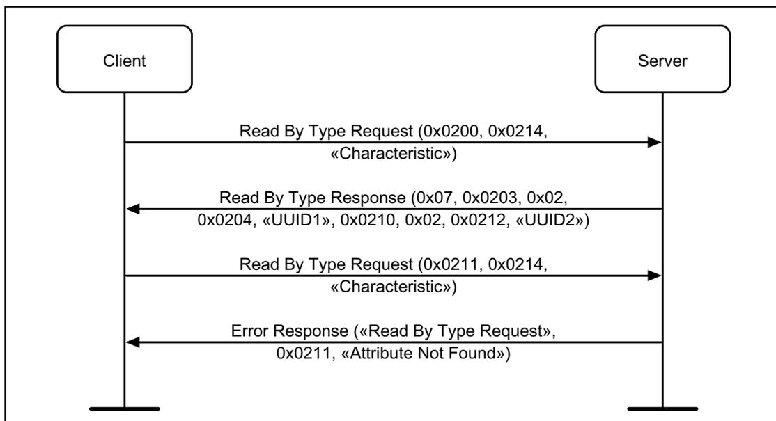
Figure 4.5: Discover All Characteristics of a Service example
