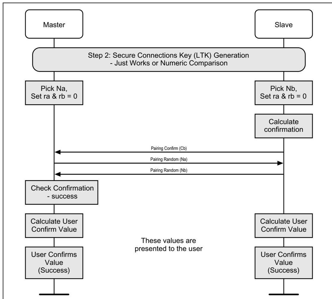
Figure C.8: Pairing Phase 2, Authentication Stage 1, Successful Numeric Comparison
