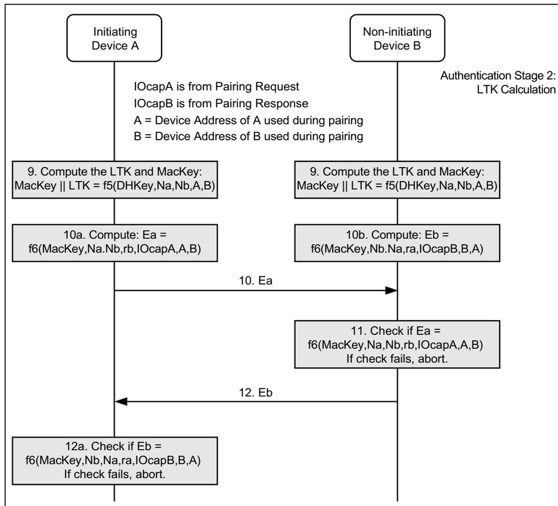
Figure 2.6: Authentication Stage 2 and Long Term Key Calculation
