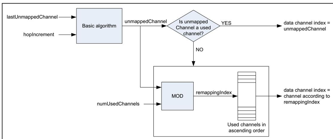
Figure 4.32: Block diagram of data Channel Selection Algorithm #1
