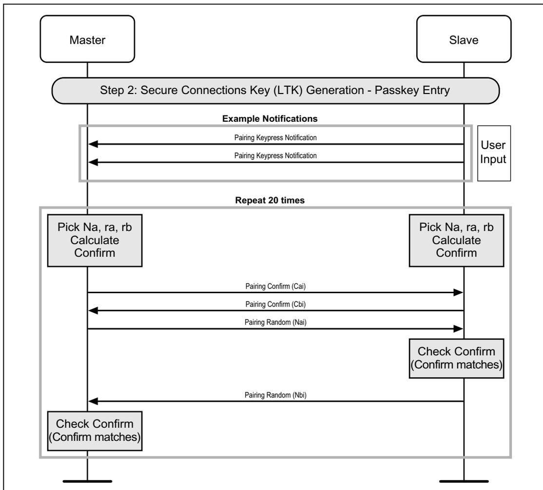
Figure C.12: Pairing Phase 2, Authentication Stage 1, Successful Passkey Entry
