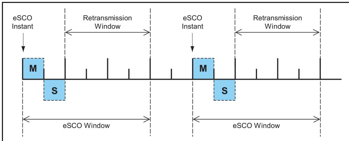
Figure 8.9: eSCO Window Details for Single-Slot Packets
